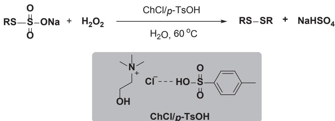
**Scheme 1** Synthesis of disulfides catalysed by acidic deep eutectic mixture.
