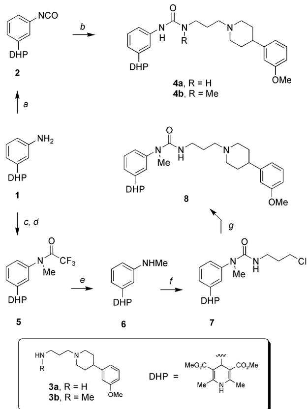
Scheme 1. Synthesis of ureas **4** and **8**: (a) COCl<sub>2</sub>, THF (100%); (b) **3a** or **3b**, CH<sub>2</sub>Cl<sub>2</sub> (60% for **4a**, 67% for **4b**); (c) (CF<sub>3</sub>CO)<sub>2</sub>O, pyridine, CH<sub>2</sub>Cl<sub>2</sub> (74%); (d) NaH, MeI, DMF (90%); (e) NaOH, EtOH (86%); (f) Cl(CH<sub>2</sub>)<sub>3</sub>NCO, CH<sub>2</sub>Cl<sub>2</sub> (75%); (g) 4-(3-methoxyphenyl)piperidine, NaI, K<sub>2</sub>CO<sub>3</sub>, MeCN (46%).
