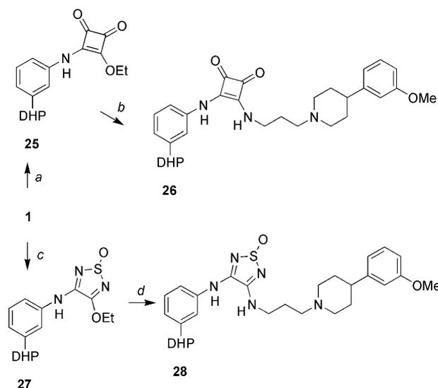
**Scheme 6.** Synthesis of heterocycles **26** and **28**: (a) 3,4-diethoxy-3-cyclobuten-1,2-dione, DMF (52%); (b) **3a**, DMF (54%); (c)  $Me_3Al$ ,  $CH_2Cl_2$ , 4,5-die-thoxythiadiazole oxide (48%); (d) **3a**, MeCN (55%).
