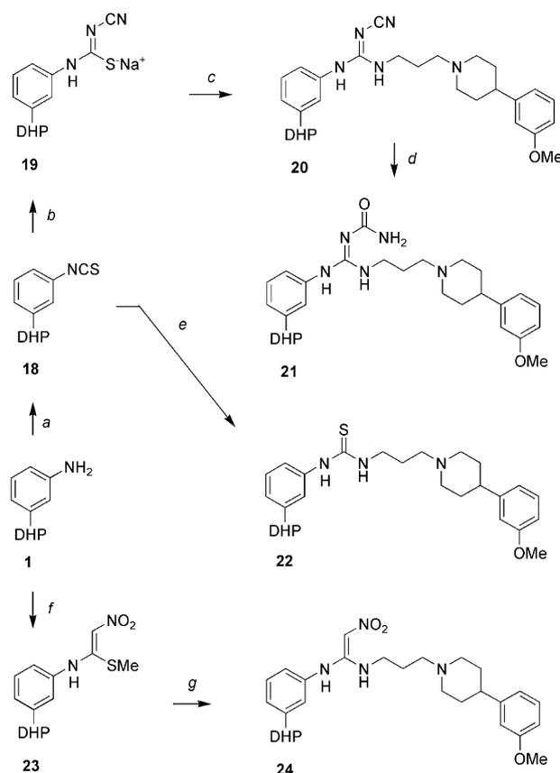
Scheme 5. Synthesis of urea replacements **20**, **21**, **22**, and **24**: (a) TCDI, DMF (75%); (b) NaNHCN, EtOH (100%); (c) **3a**, HgCl<sub>2</sub>, THF (58%); (d) **20**-HCl, storage at rt; (e) **3a**, CHCl<sub>3</sub> (100%); (f) (MeS)<sub>2</sub>CCHNO<sub>2</sub>, MeCN (77%); (g) **3a**, CH<sub>2</sub>Cl<sub>2</sub> (66%).
