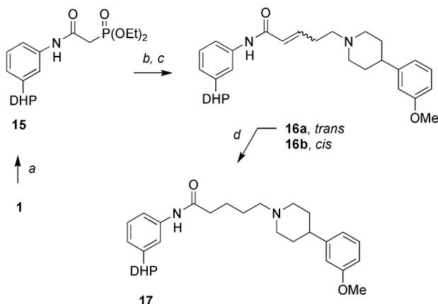
Scheme 4. Synthesis of amides **16** and **17**: (a) (EtO)<sub>2</sub>POCH<sub>2</sub>CO<sub>2</sub>H, DMAP, 2-mercaptothiazoline, DCC, CH<sub>2</sub>Cl<sub>2</sub> (80%); (b) NaH, THF; (c) acrolein, DBU, 4-(3-methoxyphenyl)piperidine, THF, (15% for **16a**, 5% for **16b**); (d) H<sub>2</sub>, 10% Pd/C, MeOH (60%).
