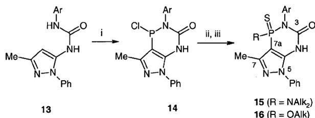
**Scheme 3** Reagents and conditions: (i)  $\text{PCl}_3$ , pyridine, r.t., 20 h; (ii) for **15**:  $\text{Alk}_2\text{NH}$ , pyridine; for **16**:  $\text{AlkOH}$ , pyridine; (iii) S, pyridine
