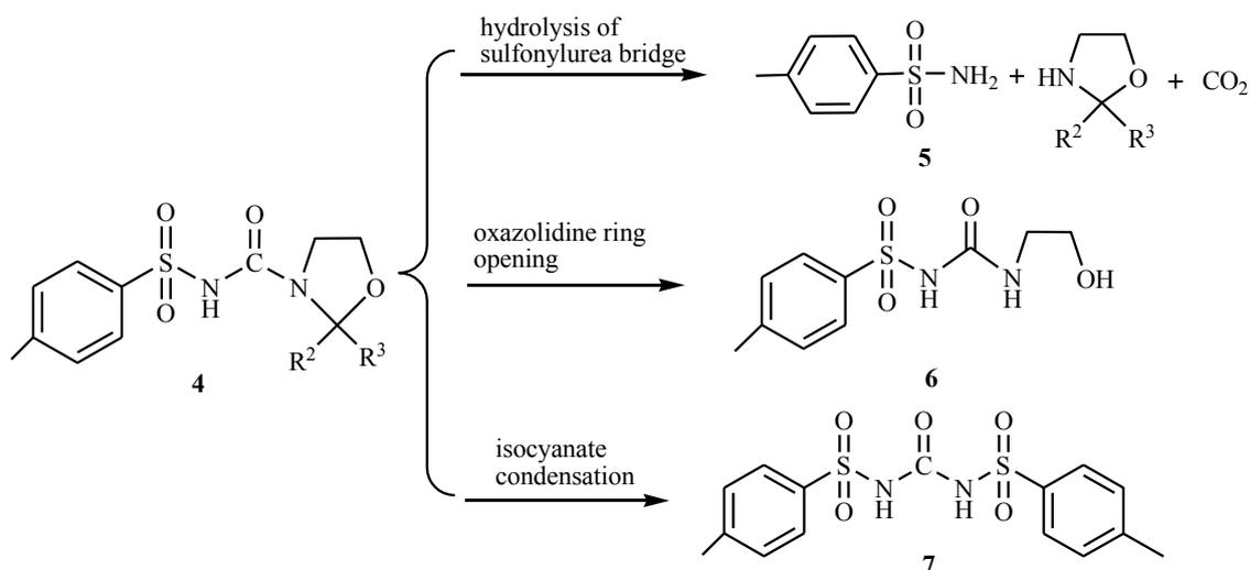
**Scheme 5.** The schematic diagram of the cleavage products
