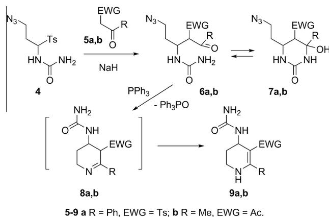
**Scheme 3.** Synthesis of 3-functionalized 4-ureido-1,2,3,4-tetrahydropyridines **9a,b** using the amidoalkylation/Staudinger/aza-Wittig sequence.
