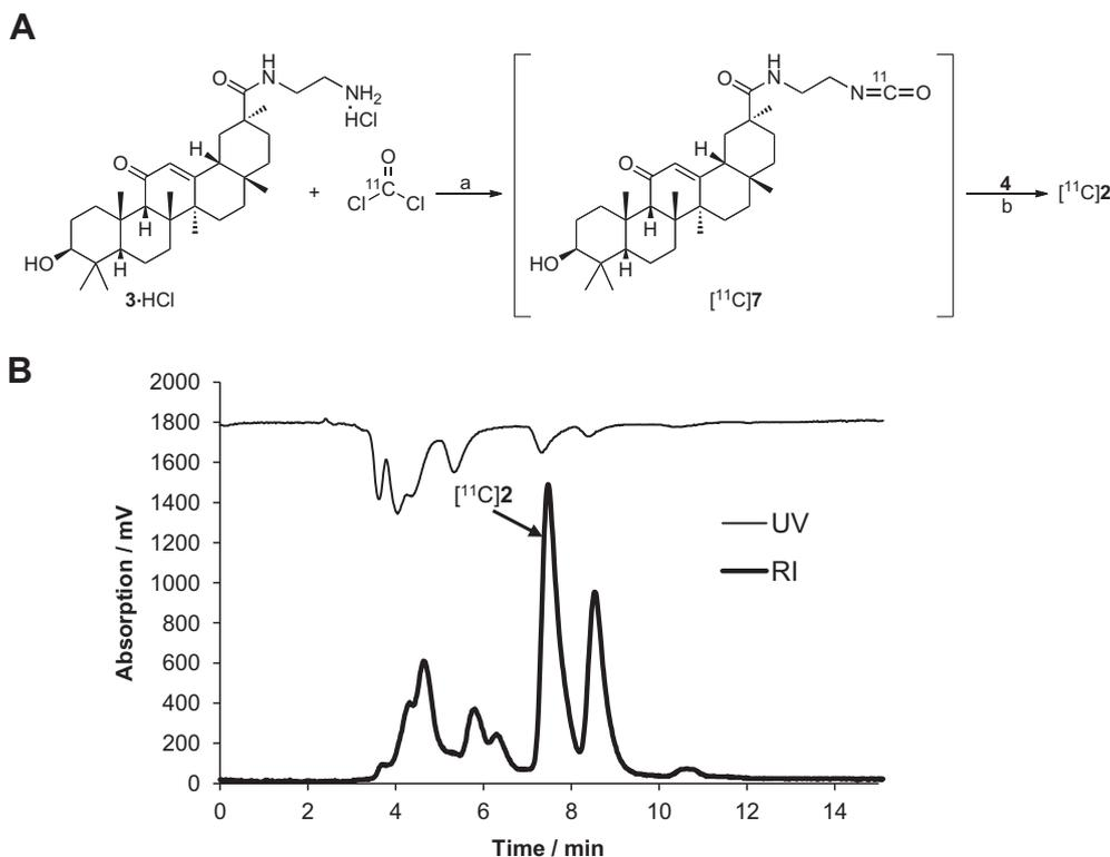
**Figure 1.** (A). Radiosynthesis from **3**-HCl: (a) THF,  $-15^\circ\text{C}$ , 1 min; (b) THF,  $60^\circ\text{C}$ , 3 min, 32.7% (incorporation of total radioactivity in the final reaction mixture). (B) HPLC chromatogram for the reaction mixture.
