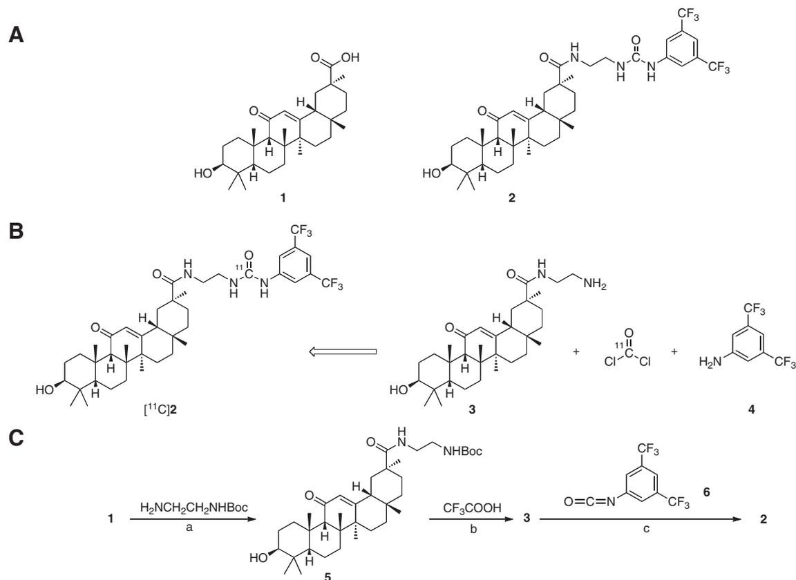
**Scheme 1.** Reagents and conditions: (A) Chemical structures of **1** and **2**; (B) retrosynthesis of  $[^{11}\text{C}]\mathbf{2}$ ; (C) syntheses of **2** and **3**: (a) *N,N'*-dicyclohexylcarbodiimide, hydroxybenzotriazole, DMF, room temperature, 10 h, 90%; (b)  $\text{CH}_2\text{Cl}_2$ , room temperature, 2 h, 65%; (c) THF, room temperature, 10 h, 76%.
