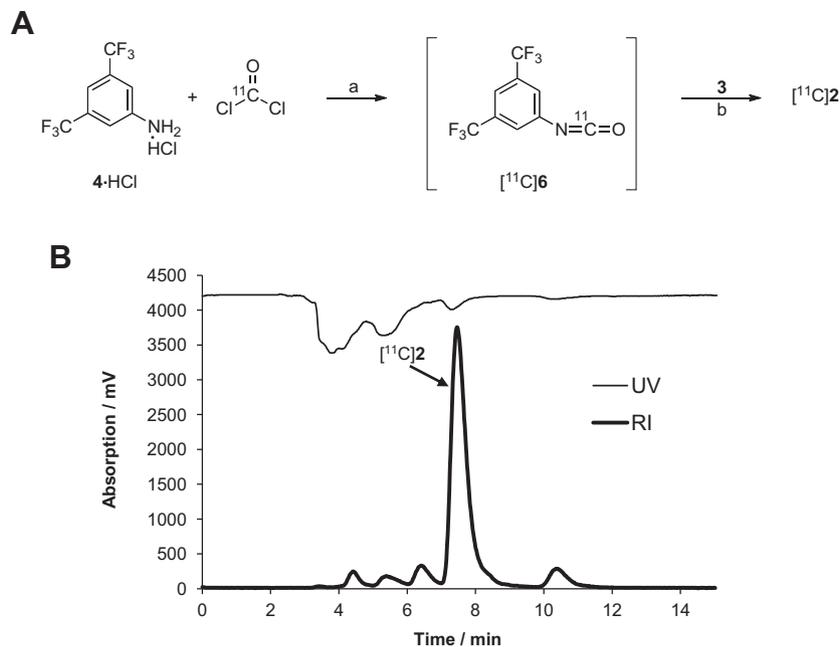
**Figure 2.** (A). Radiosynthesis from **4-HCl**: (a) THF,  $-15^{\circ}\text{C}$ , 1 min; (b) THF,  $60^{\circ}\text{C}$ , 3 min, 69.1% (incorporation of total radioactivity in the final reaction mixture). (B) HPLC chromatogram for the reaction mixture.
