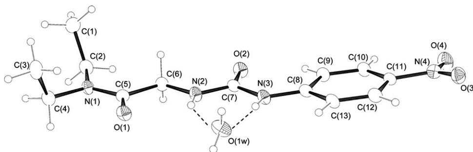
Fig. 1 ORTEP 3 view of **L2**·H<sub>2</sub>O species. Ellipsoids are drawn at 30% probability.
