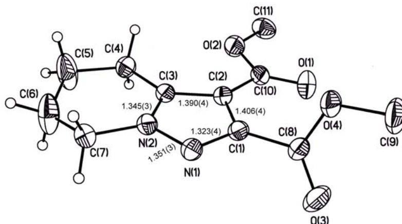
**Figure 2.** ORTEP Plots of Dimethyl 4,5,6,7-tetrahydropyrazolo-[1,5-*a*]pyridine-2,3-dicarboxylate (**11a**)
