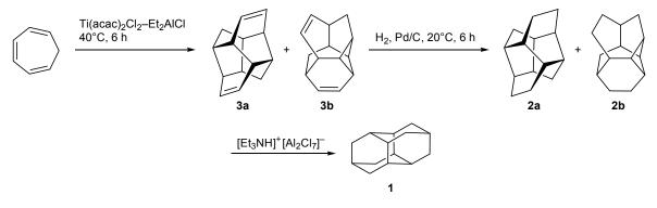
Synthesis of diamantane (1) by skeletal isomerization of a 3:2 mixture of pentacyclo[ $8.4.0.0^{3.7}.0^{4,14}.0^{6,11}$ ]tetradecane (2a) and pentacyclo[ $7.5.0.0^{2,8}.0^{5,14}.0^{7,11}$ ]tetradecane (2b)
