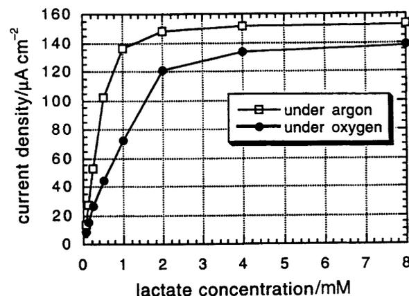
Fig. 10 Calibration curve for a typical PVP-dmo-bpy-Os lactate electrode with  $5 \mu\text{g}$  PVP-dmo-bpy-Os,  $2.25 \mu\text{g}$  LOx,  $0.73 \mu\text{g}$  PEG-400;  $6 \text{ mM}$  lactate;  $1000 \text{ rpm}$ ;  $T = 21.3^\circ\text{C}$
