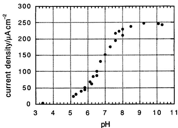
Fig. 7 pH dependence of the glucose electrooxidation current density in a typical PVP-dmo-bpy-Os based electrode with  $40 \mu\text{g}$  PVP-dmo-bpy-Os,  $18 \mu\text{g}$  GOx,  $5.8 \mu\text{g}$  PEG-400;  $20 \text{ mM}$  glucose; under argon;  $1000 \text{ rpm}$ ;  $T = 21.3^\circ\text{C}$
