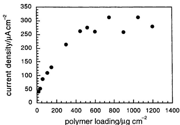
**Fig. 5** Dependence of glucose electrooxidation current densities on PVP-dmo-bpy-Os loading for electrodes with 30 wt.% GOx; 20 mM glucose; under argon; 1000 rpm;  $T = 21.3^\circ\text{C}$
