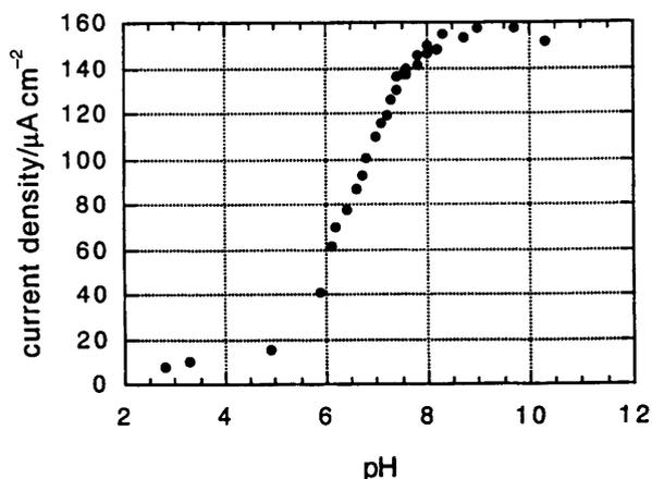
Fig. 8 pH dependence of the lactate electrooxidation current density in a typical PVP-dmo-bpy-Os based electrode with  $5 \mu\text{g}$  PVP-dmo-bpy-Os,  $2.25 \mu\text{g}$  LOx,  $0.73 \mu\text{g}$  PEG-400;  $6 \text{ mM}$  lactate; under argon;  $1000 \text{ rpm}$ ;  $T = 21.3^\circ\text{C}$
