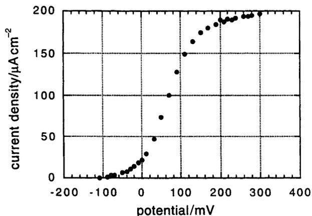
**Fig. 2** Potential dependence of the current density for a typical PVP-dmo-bpy-Os glucose electrode with 20  $\mu\text{g}$  PVP-dmo-bpy-Os, 9  $\mu\text{g}$  GOx, 2.9  $\mu\text{g}$  PEG-400; 20 mM glucose; under argon; 1000 rpm;  $T = 21.3^\circ\text{C}$
