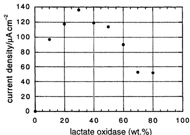
**Fig. 4** Dependence of lactate electrooxidation current densities on LOx (wt.%) for electrodes with 5  $\mu\text{g}$  PVP-dmo-bpy-Os, 0.5–12.5  $\mu\text{g}$  LOx, 10 wt.% PEG-400; 6 mM lactate; under argon; 1000 rpm;  $T = 21.3^\circ\text{C}$
