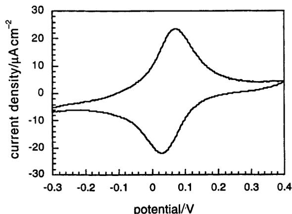
Fig. 1 Cyclic voltammogram of a typical PVP-dmo-bpy-Os glucose electrode with 40 μg PVP-dmo-bpy-Os, 18 μg GOx, 5.8 μg PEG-400; scan rate = 5 mV s<sup>-1</sup>; under air; *T* = 21.3 °C
