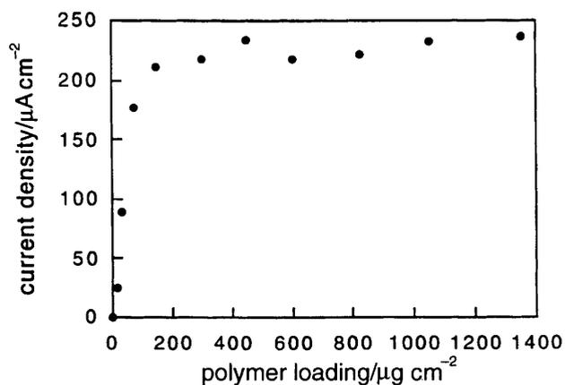
**Fig. 6** Dependence of the lactate electrooxidation current densities on PVP-dmo-bpy-Os loading for electrodes with 30 wt.% LOx; 6 mM lactate; under argon; 1000 rpm;  $T = 21.3^\circ\text{C}$
