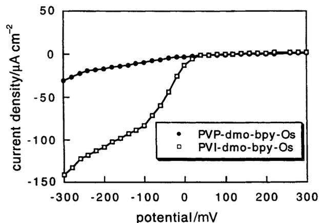
**Fig. 11** Potential dependence of the oxygen electroreduction current density for typical glucose electrodes made with PVP-dmo-bpy-Os and PVI-dmo-bpy-Os (40 µg polymer, 18 µg GOx, 5.8 µg PEG-400); in the absence of glucose; 1000 rpm;  $T = 21.3^\circ\text{C}$
