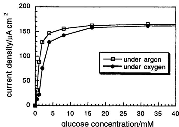
Fig. 9 Calibration curve for a typical PVP-dmo-bpy-Os glucose electrode with  $20 \mu\text{g}$  PVP-dmo-bpy-Os,  $9 \mu\text{g}$  GOx,  $2.9 \mu\text{g}$  PEG-400;  $20 \text{ mM}$  glucose;  $1000 \text{ rpm}$ ;  $T = 21.3^\circ\text{C}$
