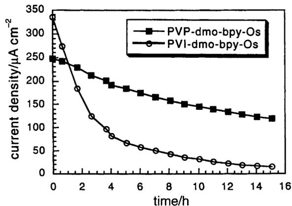
**Fig. 12** Comparison of the operational stability of typical lactate electrodes made with PVP-dmo-bpy-Os and PVI-dmo-bpy-Os (40 µg polymer, 18 µg LOx, 5.8 µg PEG-400); 6 mM lactate; under argon; 1000 rpm;  $T = 21.3^\circ\text{C}$
