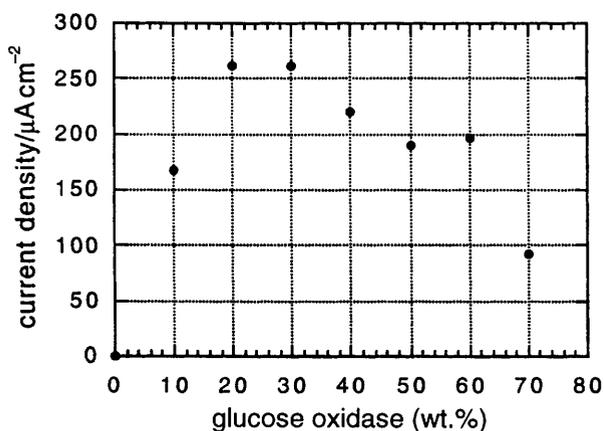
**Fig. 3** Dependence of glucose electrooxidation current densities on GOx (wt.%) for electrodes with 40  $\mu\text{g}$  PVP-dmo-bpy-Os, 4–100  $\mu\text{g}$  GOx, 10 wt.% PEG-400; 20 mM glucose; under argon; 1000 rpm;  $T = 21.3^\circ\text{C}$
