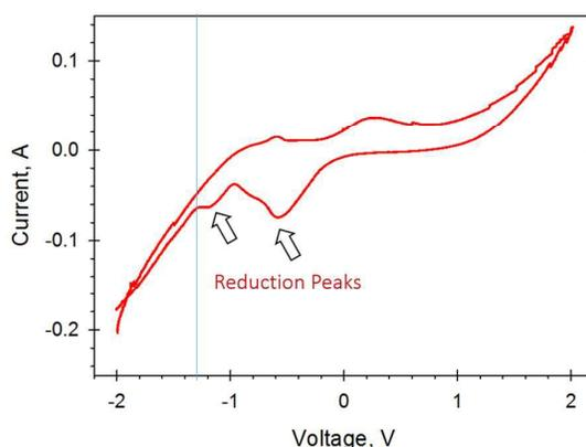
Figure 4. Cyclic voltammetry (CV) profiles from -2 / +2 V (vs. Ag/AgCl) at a scan rate of 5 mV/s on Cu10-CNT/C.
