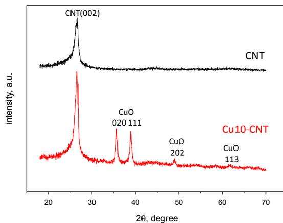
**Figure 1** X-ray diffraction patterns for Cu10-CNT electrocatalyst and of parent CNT substrate as reference.
