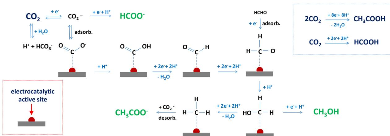
Figure 5: Schematic mechanistic pathway for the electrocatalytic production of formic acid, acetic acid and methanol on Cu<sub>10</sub>-CNT/C.
