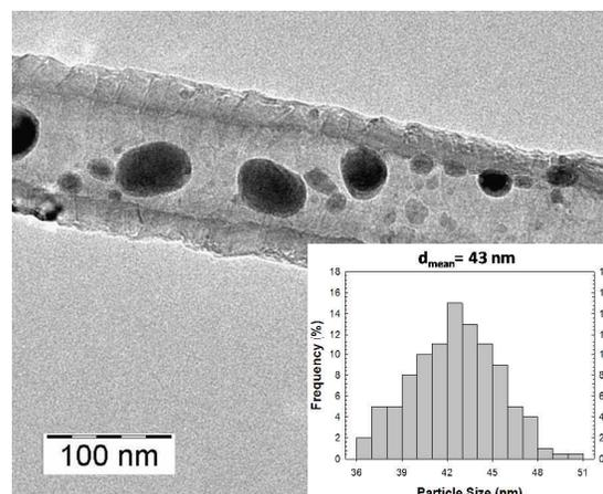
**Figure 2** TEM image of Cu10-CNT sample with the estimated particle distribution.
