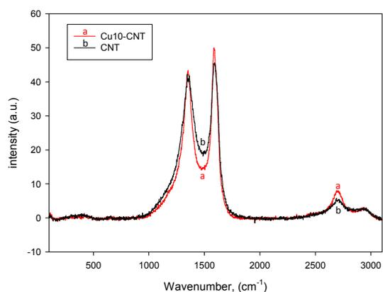
Figure 3. Raman spectra of pure CNTs and Cu10-CNT sample.
