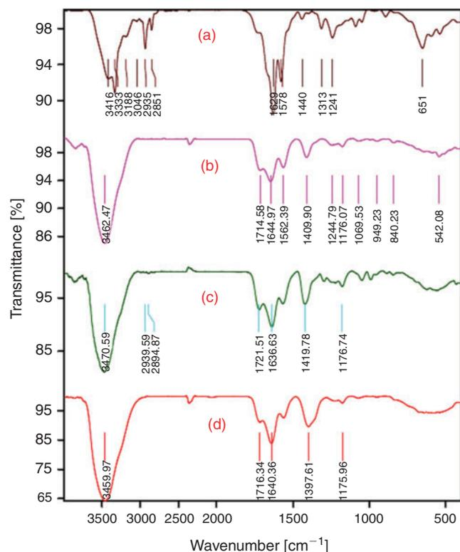
**Fig. 2.** FT-IR spectra of (a) peptide powder, (b) peptide nanofibre, (c) peptide nanofibres decorated with Cu nanoparticles, and (d) peptide nanofibres decorated with Ni nanoparticles.
