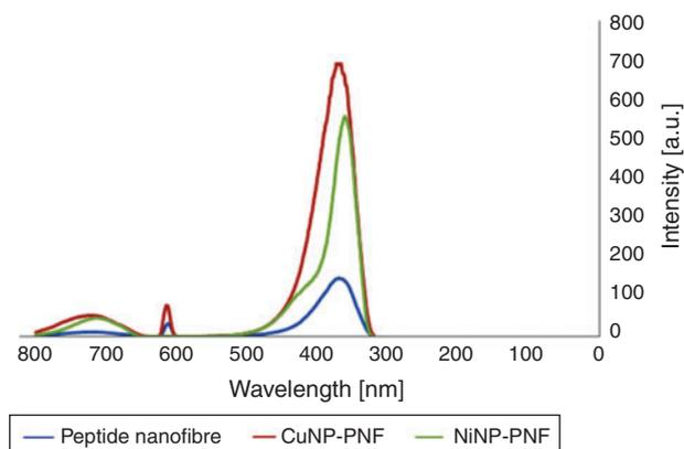
**Fig. 5.** Fluorescence spectra of peptide nanofibre and NiNP-PNF and CuNP-PNF.
