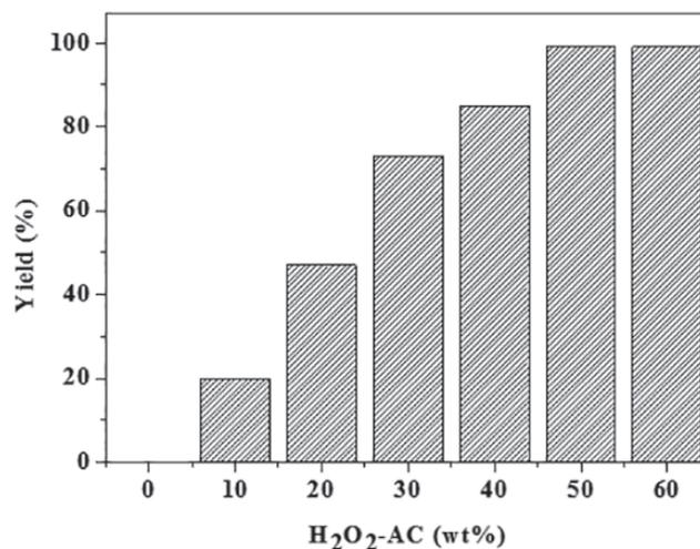
**Fig. 2** Effects of amount of H<sub>2</sub>O<sub>2</sub>-AC on the yield of the model reaction in 3 h.
