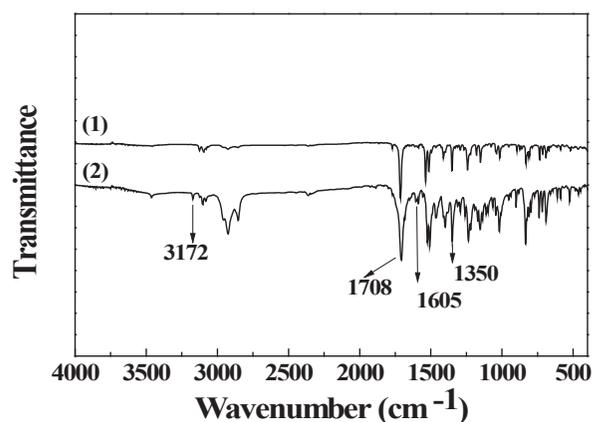
**Fig. 1** FTIR spectra of ACs (1) before  $\text{H}_2\text{O}_2$ -treatment (2) after  $\text{H}_2\text{O}_2$ -treatment.
