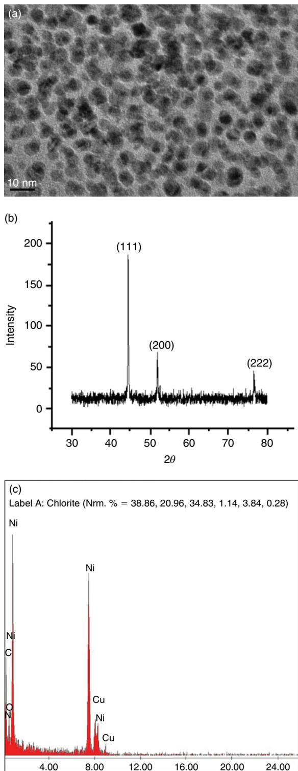
**Fig. 1.** (a) TEM image of PEG-stabilized Ni nanoparticles. (b) X-ray diffraction pattern of PEG-Ni nanoparticles. (c) EDAX data of PEG-Ni nanoparticles.
