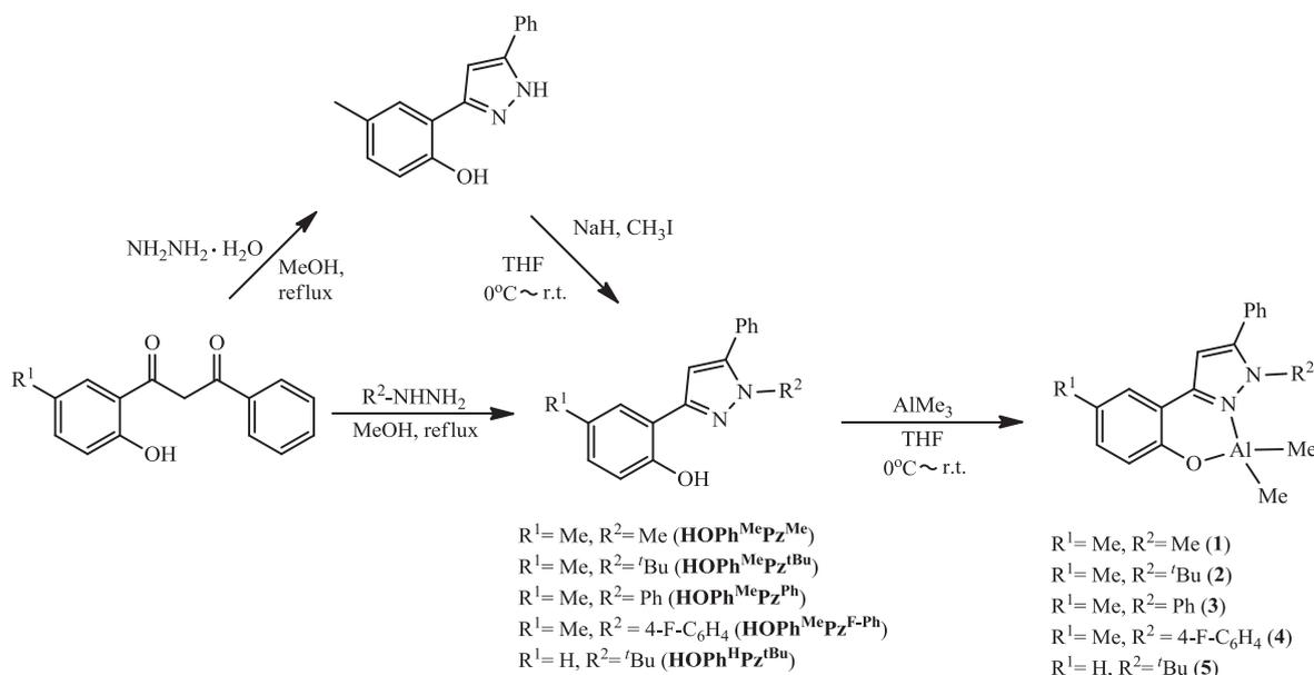
**Scheme 1.** Synthesis of aluminium pyrazolyl-phenolate complexes **1–5**.
