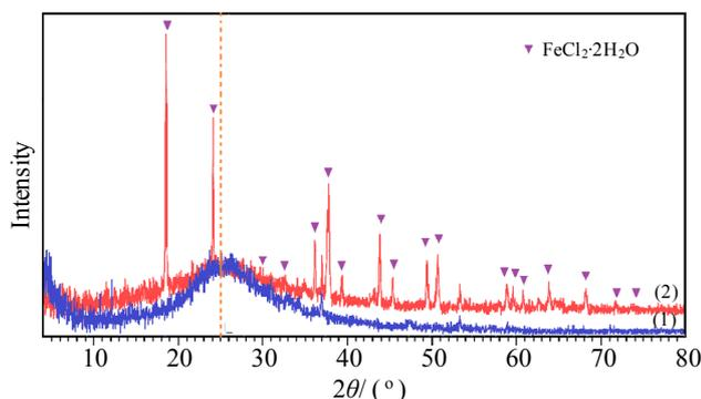
Fig. 3. XRD patterns of RiHA (1) and FeCl<sub>2</sub>·2H<sub>2</sub>O-RiHA (2).
