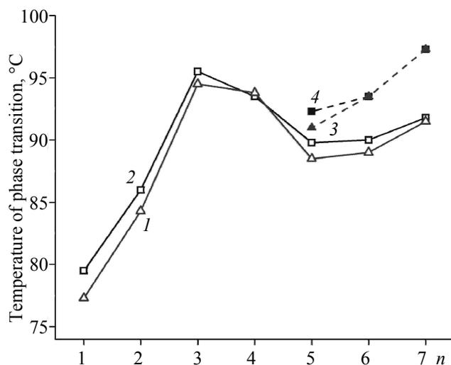
Plot of temperatures of phase transitions in glycerol ethers **1a–1g** as a function of the number of carbon atoms (*n*) in the linear hydrocarbon substituent R. Melting points: (1) scalemic samples (*ee*  $\geq$  97%); (2) racemates; temperature of transition to isotropic state: (3) scalemic samples; (4) racemates.
