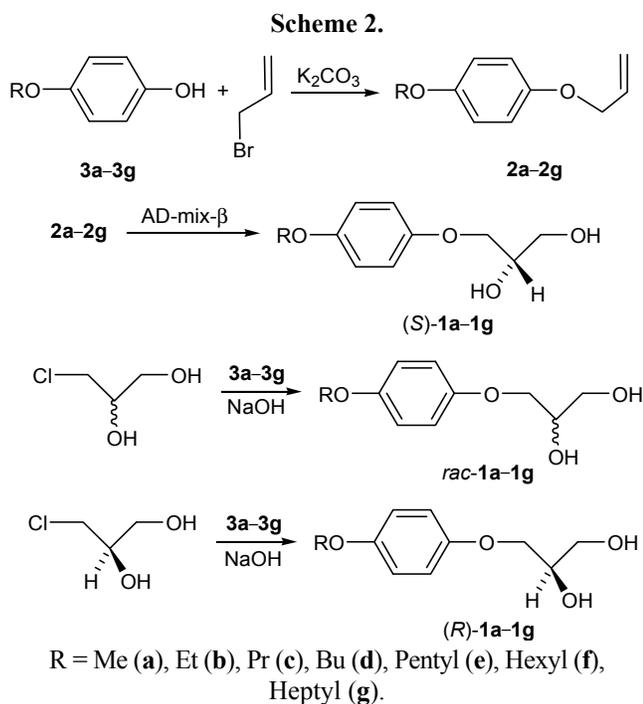
dihydroxylation afforded the corresponding scalemic diols *scal*-**1a–1g** with a moderate enantiomer excess (*ee* 86–92%). The length of the alkoxy substituent in aryl allyl ethers **2a–2g** located far from the prochiral double bond virtually did not affect the enantioselectivity of the reaction.
