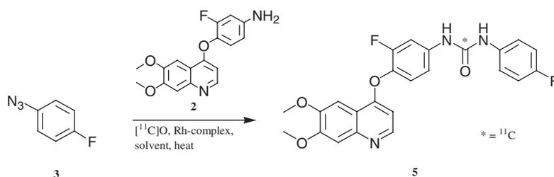
**Scheme 2.** Rhodium-mediated carbonylative cross-coupling between 4-fluoro-phenylazide and an aniline **2** using  $[^{11}\text{C}]\text{CO}$ .
