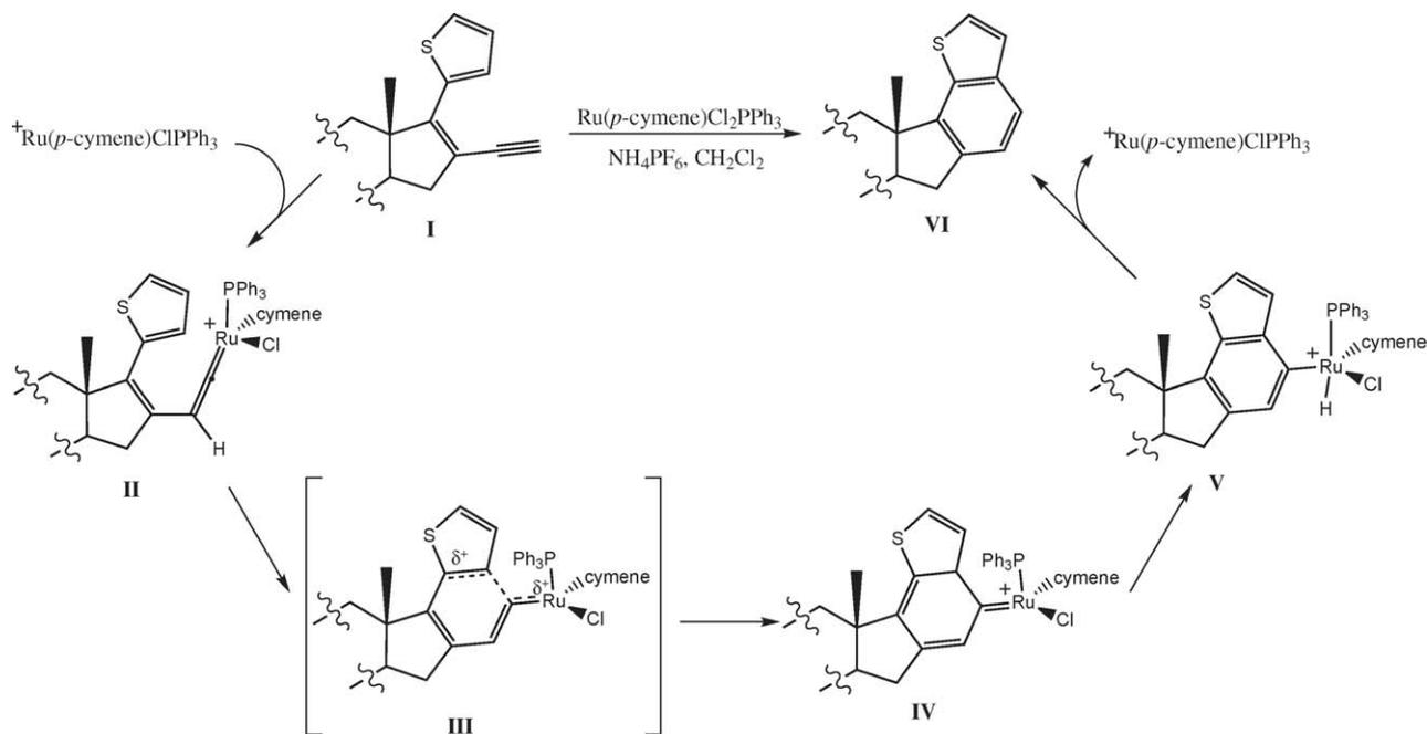
Scheme 4. Proposed mechanism for the ruthenium catalyzed heteroaryl-ene-yne cyclization according to Merlic and Pauly [22].
