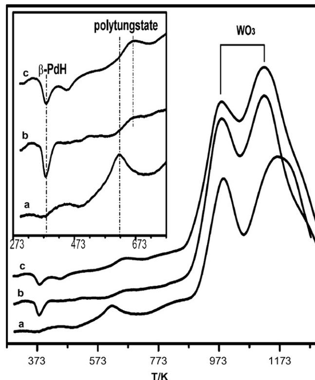
Fig. 2. H<sub>2</sub>-TPR spectra of Pd/WO<sub>3</sub>-ZrO<sub>2</sub> catalysts prepared with different Pd precursors: (a) PdCl<sub>2</sub>; (b) Pd(NH<sub>3</sub>)<sub>2</sub>Cl<sub>2</sub>; (c) Pd(CH<sub>3</sub>COO)<sub>2</sub>.
