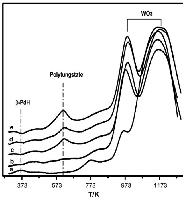
Fig. 1. H<sub>2</sub>-TPR spectra of Pd/WO<sub>3</sub>-ZrO<sub>2</sub> with different Pd loadings: (a) 0%; (b) 0.5%; (c) 1%; (d) 1.5%; (e) 2%.
