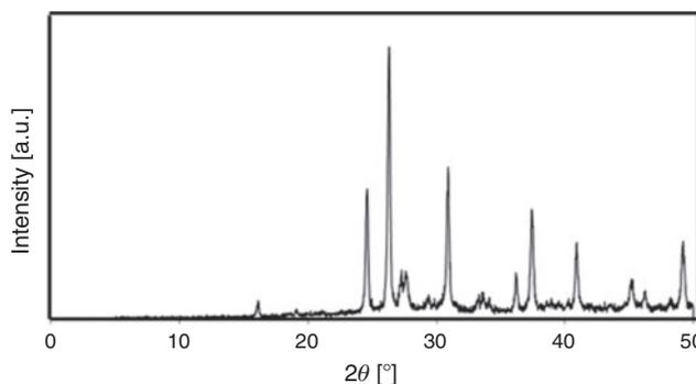
Fig. 1. Powder X-ray diffraction patterns of as-synthesized pollucite.
