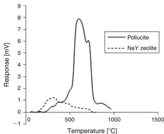
Fig. 2. Comparison of the temperature-programmed desorption profiles of adsorbed  $\text{CO}_2$  onto the synthesized pollucite and NaY zeolite.
