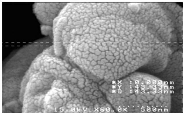
Fig. 3. Scanning electron microscopy image of synthesized pollucite.
