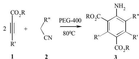
**Scheme 1.** Synthesis of high polysubstituted aniline derivatives.
