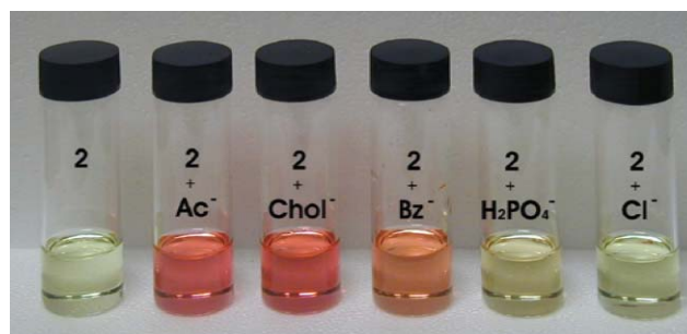
Fig. 1 Colour changes observed on addition of 1 eq. of anion (as a tetrabutylammonium salt; sodium for cholate) to a DMSO solution of receptor 2 .
