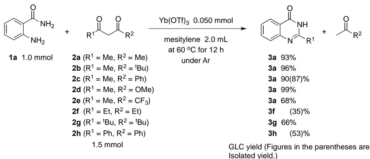
**Scheme 2.** Yb(OTf)<sub>3</sub>-catalyzed synthesis of 2-substituted 4(3*H*)-quinazolinones **3** from 2-aminobenzamide **1a** and 1,3-diketones (or β-ketoester) **2**
