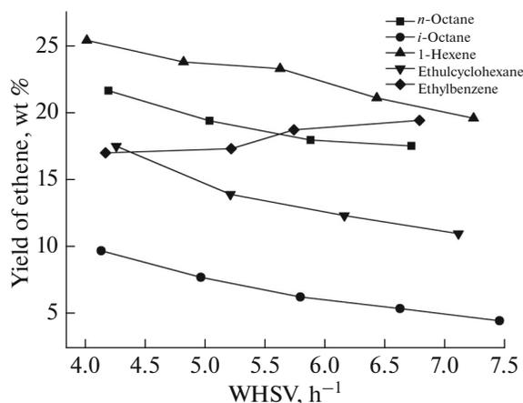
Fig. 4. Effect of WHSV on ethene yield (reaction temperature, 660°C; S/O ratio, 0.36).
