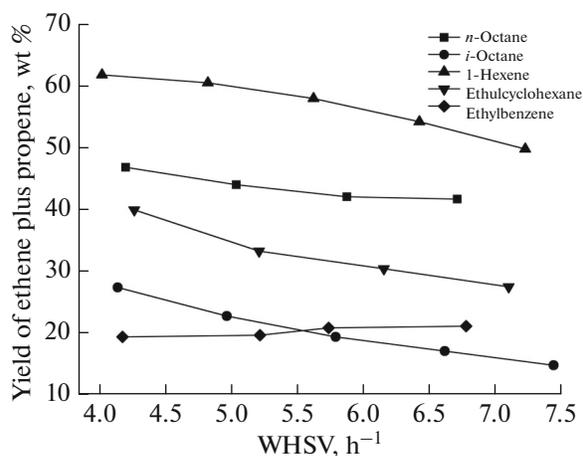
Fig. 6. Effect of WHSV on the yield of ethene plus propene (reaction temperature, 660°C; S/O ratio, 0.36).
