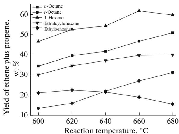
Fig. 3. Effect of reaction temperature on the yield of ethene plus propene (WHSV,  $4.2 \text{ h}^{-1}$ ; S/O ratio, 0.36).
