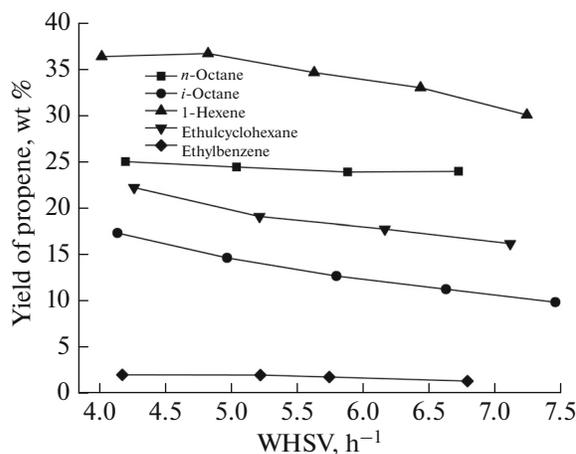
Fig. 5. Effect of WHSV on propene yield (reaction temperature, 660°C; S/O ratio, 0.36).
