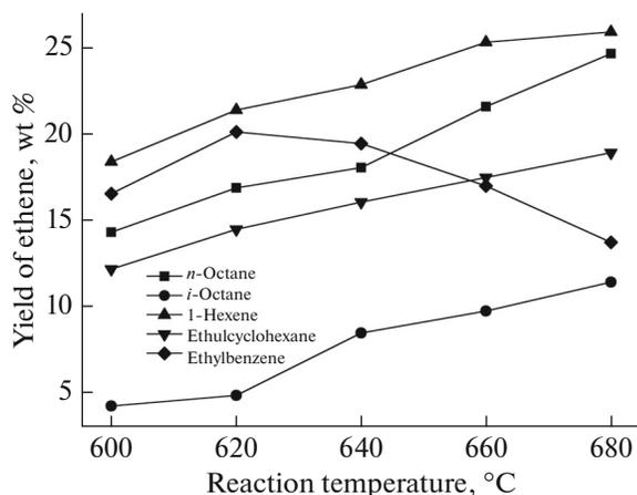
Fig. 1. Effect of reaction temperature on ethene yield (WHSV, 4.2 h<sup>-1</sup>; S/O ratio, 0.36).
