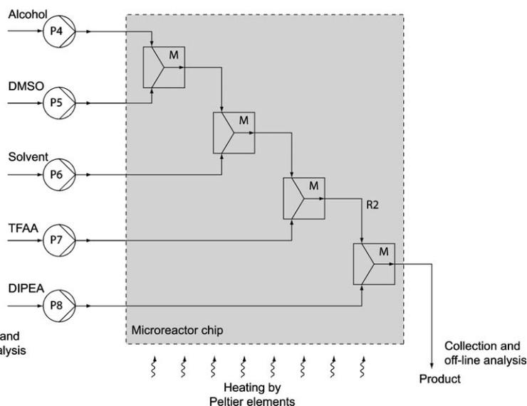
Figure 1. Microreactor setups 1 and 2, with relevant reactor volumes designated 'R1' and 'R2'.
