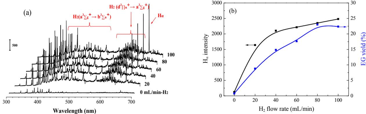
**Fig. 2.** OES of the CH<sub>3</sub>OH/H<sub>2</sub> non-equilibrium plasma (a), and the correlation between the intensity of the H<sub>α</sub> line and EG yield (b) at different flow rates of H<sub>2</sub>. Reaction conditions: CH<sub>3</sub>OH gas flow rate = 11.1 mL/min, pressure = 0.1 MPa, discharge frequency = 12.0 kHz, input power = 11 W, discharge voltage = 16.8 kV, temperature = 300 °C.
