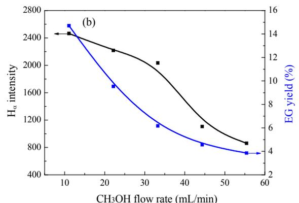
**Fig. 4.** OES of the  $CH_3OH/H_2$  non-equilibrium plasma (a) and the correlation between the intensity of the  $H_\alpha$  line and EG yield (b) at different  $CH_3OH$  gas flow rates. Reaction conditions:  $H_2$  flow rate = 80 mL/min, pressure = 0.1 MPa, discharge frequency = 12.0 kHz, input power = 17 W, discharge voltage = 16.8 kV, temperature = 300 °C.
