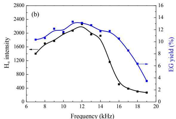
**Fig. 3.** OES of the  $CH_3OH/H_2$  non-equilibrium plasma (a) and the correlation between the intensity of the  $H_\alpha$  line and EG yield (b) at different discharge frequencies. Reaction conditions:  $CH_3OH$  gas flow rate = 11.1 mL/min,  $H_2$  flow rate = 60 mL/min, pressure = 0.1 MPa, input power = 17 W, discharge voltage = 16.8 kV, temperature = 300 °C.
