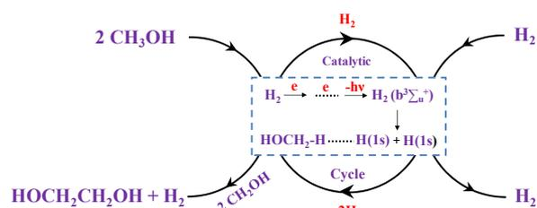
**Fig. 6.** Schematic of  $\text{H}_2$  catalytic cycle in the EG synthesis with  $\text{CH}_3\text{OH}/\text{H}_2$  plasma.
