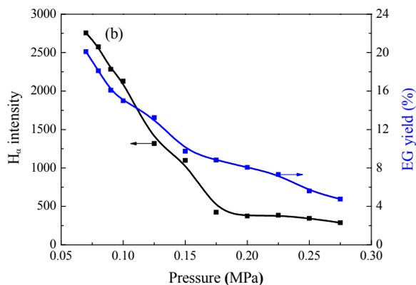
**Fig. 5.** OES of the  $\text{CH}_3\text{OH}/\text{H}_2$  non-equilibrium plasma (a) and the correlation between the intensity of the  $\text{H}_\alpha$  line and EG yield (b) at different pressures. Reaction conditions:  $\text{CH}_3\text{OH}$  gas flow rate = 11.1 mL/min,  $\text{H}_2$  flow rate = 80 mL/min, discharge frequency = 12.0 kHz, input power = 17 W, discharge voltage = 16.8 kV, temperature = 300 °C.
