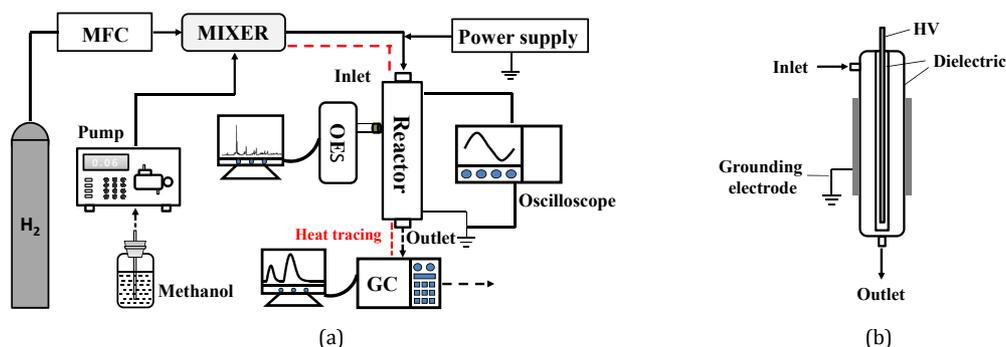
Fig. 1. Schematic of the experimental setup (a) and the reactor structure (b).
