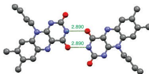
**Fig. 3.** X-Ray crystal structure of **7c** showing weak hydrogen bonding.
