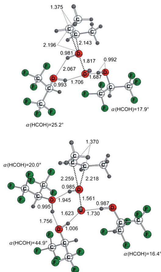
**Figure 1.** Catalysis of (*Z*)-2-butene epoxidation, effected by two (top) and three (bottom) molecules of HFIP, through hydrogen-bonding networks (from Ref. [3b]).
