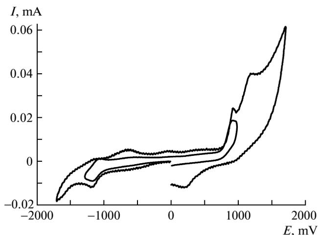
**Fig. 1.** Cyclic voltammogram of free base of porphyrin V in DMF at a potential sweep rate of 100 mV/s (Pt, porphyrin concentration  $10^{-3}$  M, *n*-Bu<sub>4</sub>NBF<sub>4</sub>, Ag/AgCl).
