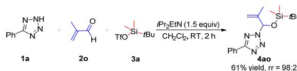
**Scheme 2** Silylation reaction of  $\alpha,\beta$ -unsaturated aldehyde **2o**.
