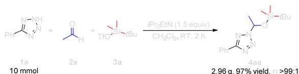
and TBSOTf **3a** proceeded well at RT for 2 h, giving the desired 2,5-disubstituted tetrazole hemiaminal silyl ether **4aa** in 2.96 g without any loss of yield and regioselectivity.
