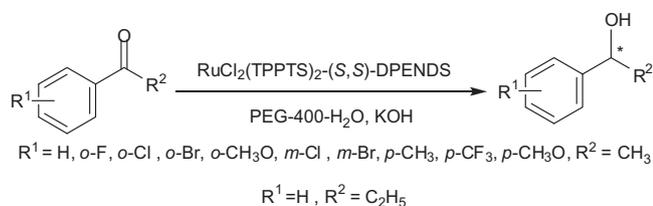
**Figure 2.** Asymmetric hydrogenation of aromatic ketones.
