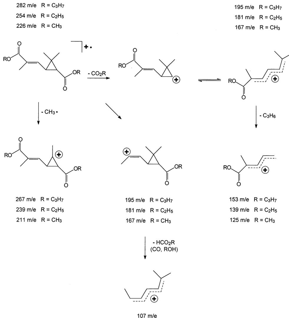
Fig. 5. Main fragmentations of dimethyl- (CH<sub>3</sub>), diethyl- (C<sub>2</sub>H<sub>5</sub>) and dipropyl- (C<sub>3</sub>H<sub>7</sub>) *trans*-(E)-chrysanthemumdicarboxylates (*trans*-(E)-CDCA).
