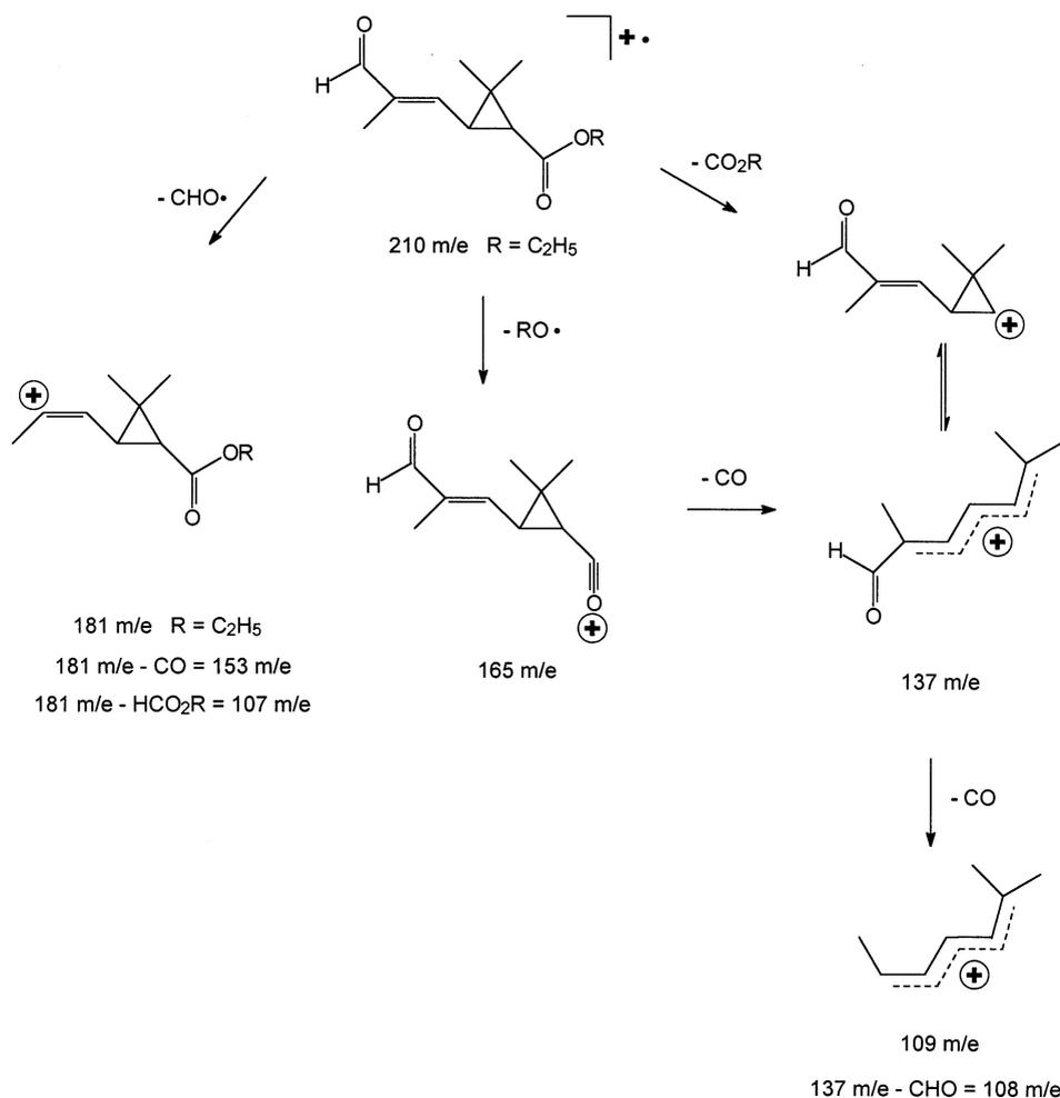
Fig. 3. Main fragmentations of the aldehyde (*cis*-/*trans*-(E)-CHO]-CA-Et) formed as an intermediate from the SeO<sub>2</sub> oxidation of the isobutenyl methyl group of *cis*-/*trans*-CA-Et.
