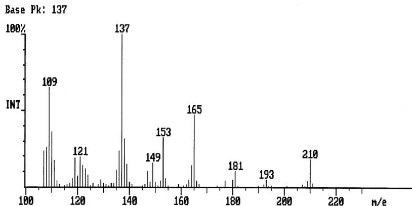
Fig. 4. ITD-mass spectra (full scan 107–220 m/e) showing the main fragmentations of the aldehyde (*cis-/trans-[(E)-CHO]-CA-Et*) indicated in Fig. 3.
