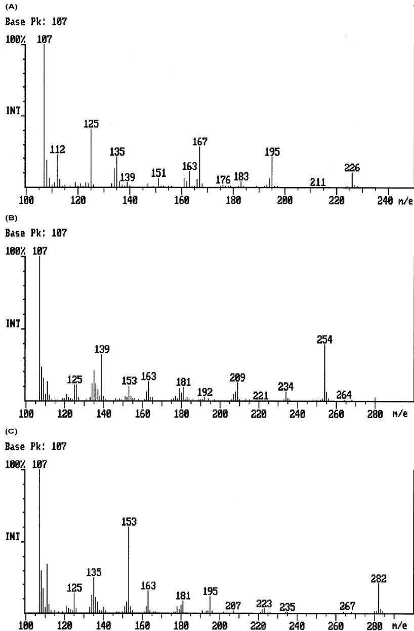
Fig. 6. ITD-mass spectra of (A) dimethyl-, (B) diethyl- and (C) dipropyl *trans*-(*E*)-chrysanthemumdicarboxylates (full scan 107–282 m/e) obtained by chemical synthesis showing main fragmentations indicated in Fig. 5.
