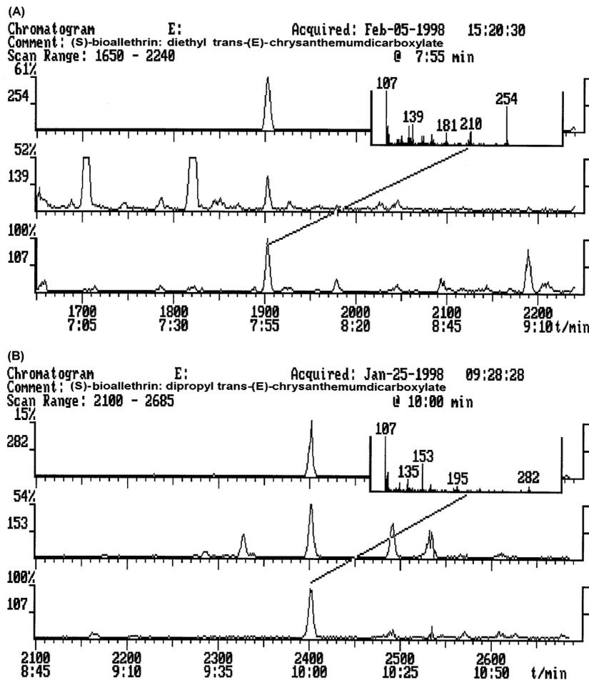
Fig. 8. Mass chromatograms (full scan) of a real 24-h urine sample from a pest control operator exposed to (*S*)-bioallethrin: *trans*-(E)-CDCA ( $204 \mu\text{g/l}$ ) derivatized as (A) diethyl and (B) dipropyl ester. Major ion fragments and retention times are virtually identical to those of the corresponding *trans*-(E)-CDCA standard given in Figs. 6 and 7. Within the limit of detection, the epimeric *cis*-(E)-CDCA is not present in the urine.
