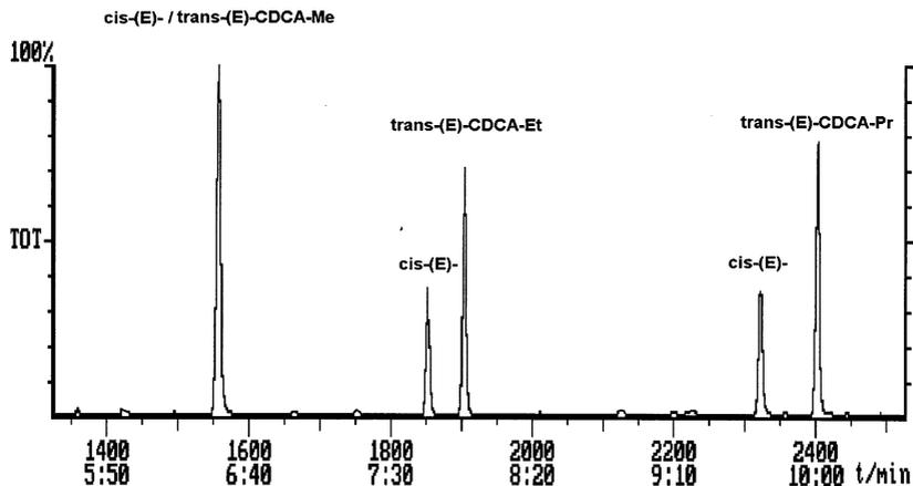
Fig. 7. Total ion chromatogram of the formed CDCA derivatives of standard solutions separated on a DB 5 ms column (standard solution containing 100  $\mu\text{g}/\text{ml}$  of each diastereomere).
