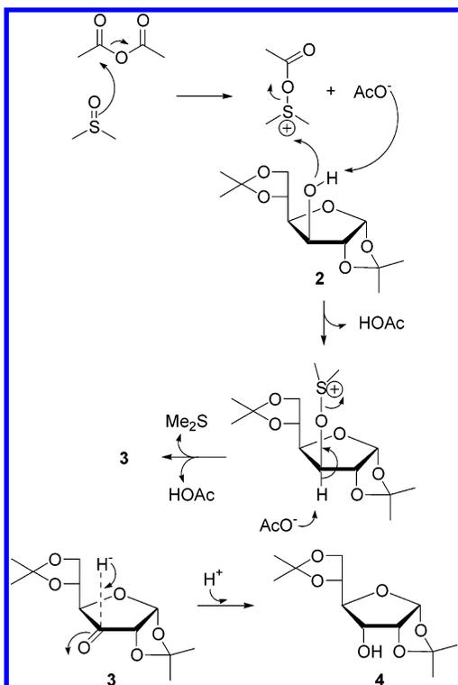
**Figure 2.** Mechanism of oxidation with DMSO/Ac<sub>2</sub>O followed by reduction.
