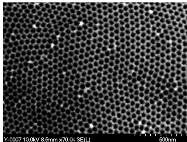
Fig. 1. FE-SEM image of surface of PAA template prepared in 1:1 sulfuric/oxalic acid mixture at 26 V and 5 °C.
