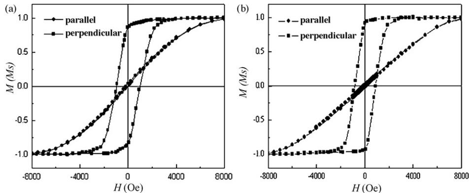
**Fig. 6.** Hysteresis loops of Co nanowires electrodeposited from aqueous solution containing  $120 \text{ g L}^{-1} \text{ CoSO}_4 \cdot 7\text{H}_2\text{O}$  and  $45 \text{ g L}^{-1} \text{ H}_3\text{BO}_3$  (a), from the electrolyte containing EMIC, anhydrous  $\text{CoCl}_2$  and ethylene glycol = 2:1:18 (by molar) (b).
