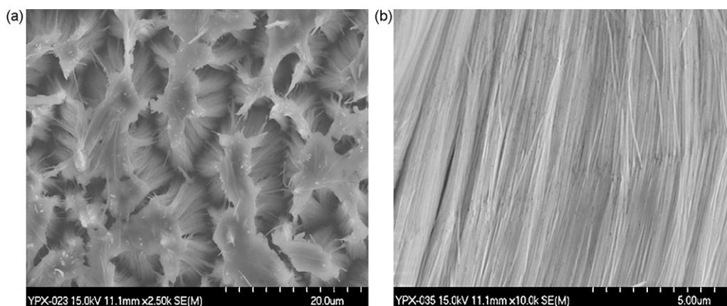
**Fig. 3.** FE-SEM images of surface (a) and cross-sectional (b) morphology of Co nanowires with alumina partially removed using 0.5 M NaOH solution.
