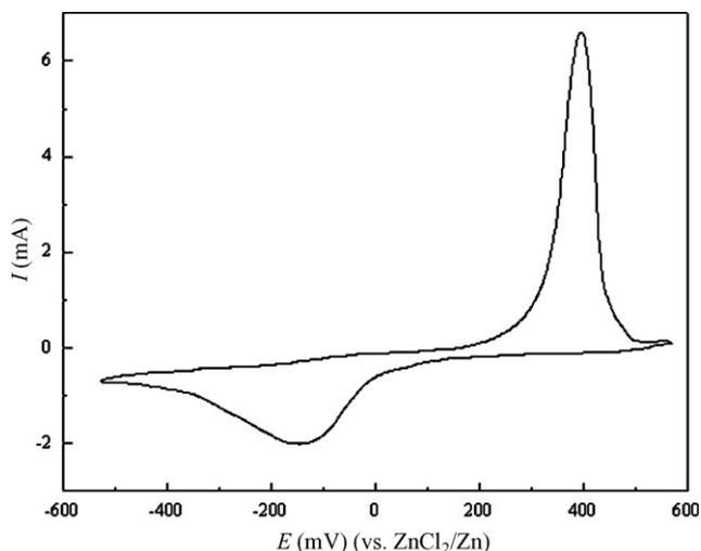
**Fig. 2.** Cyclic voltammogram for EMIC–CoCl<sub>2</sub>–ethylene glycol (2:1:18) (by molar) on Pt electrode at 80 °C. Scan rate was 50 mV/s. Electrode area was 0.5 cm<sup>2</sup>.
