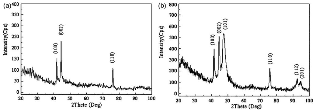
**Fig. 5.** X-ray diffraction patterns of Co nanowires from aqueous solution containing  $120 \text{ g L}^{-1} \text{ CoSO}_4 \cdot 7\text{H}_2\text{O}$  and  $45 \text{ g L}^{-1} \text{ H}_3\text{BO}_3$  (a), from the electrolyte containing EMIC, anhydrous  $\text{CoCl}_2$  and ethylene glycol = 2:1:18 (by molar) (b).
