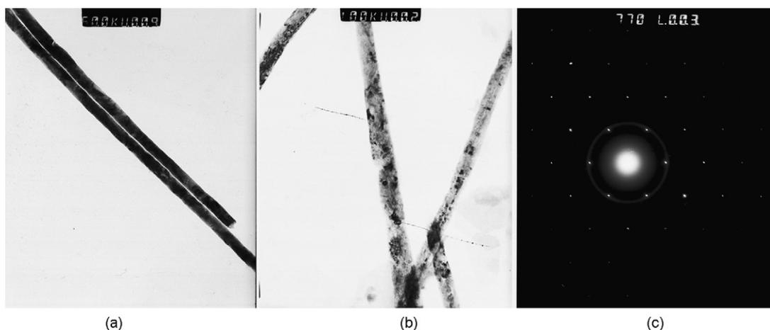
**Fig. 4.** TEM images of Co nanowires from the electrolyte containing EMIC, anhydrous CoCl<sub>2</sub> and ethylene glycol = 2:1:18 (by molar) (a), from an aqueous electrolyte containing 120 g L<sup>-1</sup> CoSO<sub>4</sub>·7H<sub>2</sub>O and 45 g L<sup>-1</sup> H<sub>3</sub>BO<sub>3</sub> (b) and selected area electron diffraction of Co nanowire electrodeposited from mixture of EMIC ionic liquid and ethylene glycol (c).
