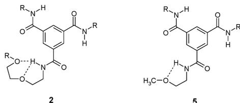
Fig. 6 Proposed folding back of ethylene glycol residues in compounds **2** and **5**.
