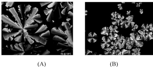
**Fig. 1** POM images under crossed polarisers of the texture of compound 2 at 138 °C (A) and of the texture of compound 5 growing from the isotropic liquid (B).
