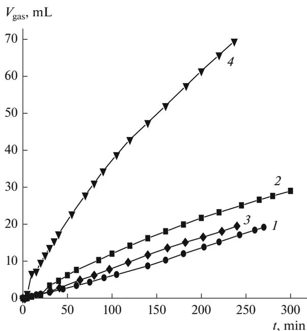
**Fig. 3.** Kinetics of gas consumption in cyclohexene oxidation by oxygen in the presence of  $\text{SiO}_2$ -supported  $\text{MoO}_3$  catalysts **II-Mo** (20 mg, curves 1 and 2; 40 mg, curve 4) and **III-Mo** (40 mg, curve 3) at  $60^\circ\text{C}$ . The compositions of initial mixtures for curves 1–4 corresponds to experiments nos. 1–4 in Table 3.
