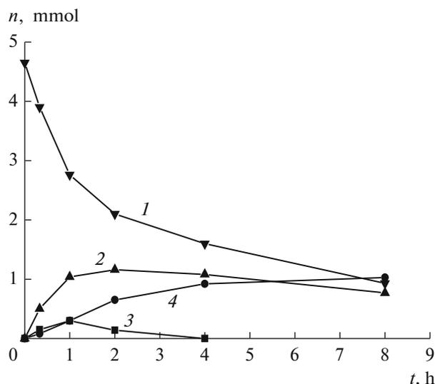
Fig. 2. Kinetics of cyclohexene (**1**) consumption and accumulation of the products of oxidation of 2-cyclohexenyl hydroperoxide (**2**), 2-cyclohexen-1-ol (**3**) and 2-cyclohexen-1-on (**4**). Reaction conditions: 1.7 mg (8.5  $\mu$ mol) Cu(OAc)<sub>2</sub> · H<sub>2</sub>O, 15 mg (0.092 mmol) NHPI, 4.65 mmol (**1**), 2 mL CH<sub>3</sub>CN, 60°C.
