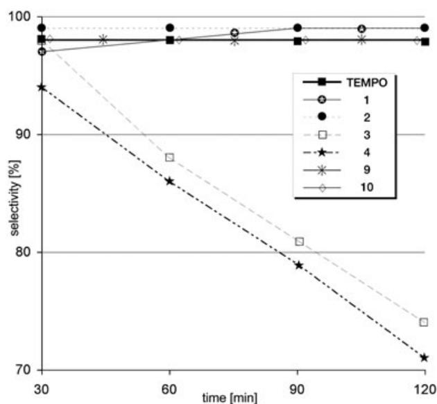
**Figure 3.** Oxidation of 1-octanol to octanal with BAIB. Selectivity profiles for reactions mediated by fluoros-tagged TEMPO radicals.
