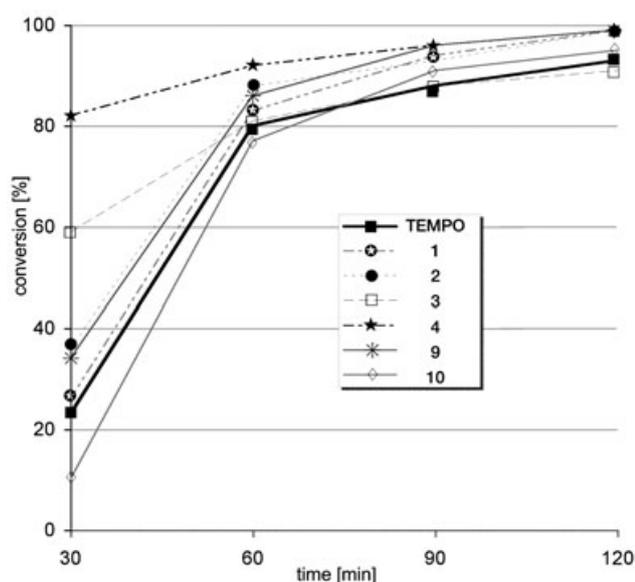
**Figure 2.** Oxidation of 1-octanol to octanal with BAIB. Conversion profiles for reactions mediated by fluoros-tagged TEMPO radicals.
