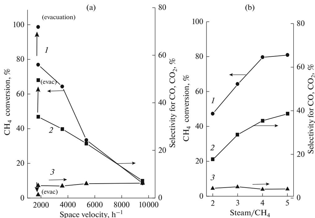
Fig. 2. Dependence of (1) methane conversion and selectivity for (2) CO<sub>2</sub> and (3) CO on (a) the feed space velocity at a steam/methane ratio of 3 and (b) the steam/methane ratio at a space velocity of 3600 h<sup>-1</sup>. *T* = 823 K.
