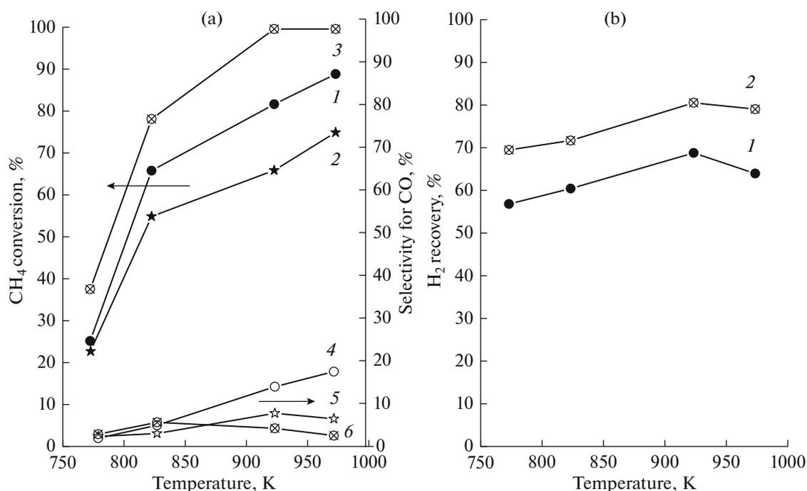
**Fig. 1.** (a) Temperature dependence of (1–3) methane conversion and (4–6) CO selectivity at a feed space velocity of  $3600 \text{ h}^{-1}$  and steam/methane = 3 (1, 4) with  $\text{H}_2$  withdrawal (sweep-gas flow rate  $150 \text{ cm}^3/\text{min}$ ), (2, 5) without  $\text{H}_2$  withdrawal, and (3, 6) with permeate evacuation used instead of sweep gas. (b) Influence of temperature on the  $\text{H}_2$  recovery through the membrane using (1) sweep gas and (2) permeate evacuation.
