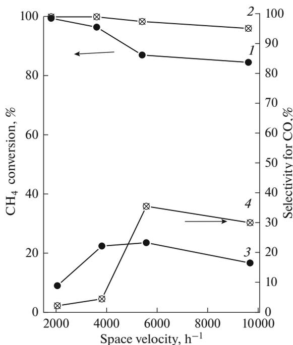
Fig. 3. Influence of feed space velocity on (1, 2) methane conversion and (3, 4) CO selectivity at  $T = 973$  K and a steam/methane ratio of 3 in experiments with (1, 3) sweep gas and (2, 4) permeate evacuation.
