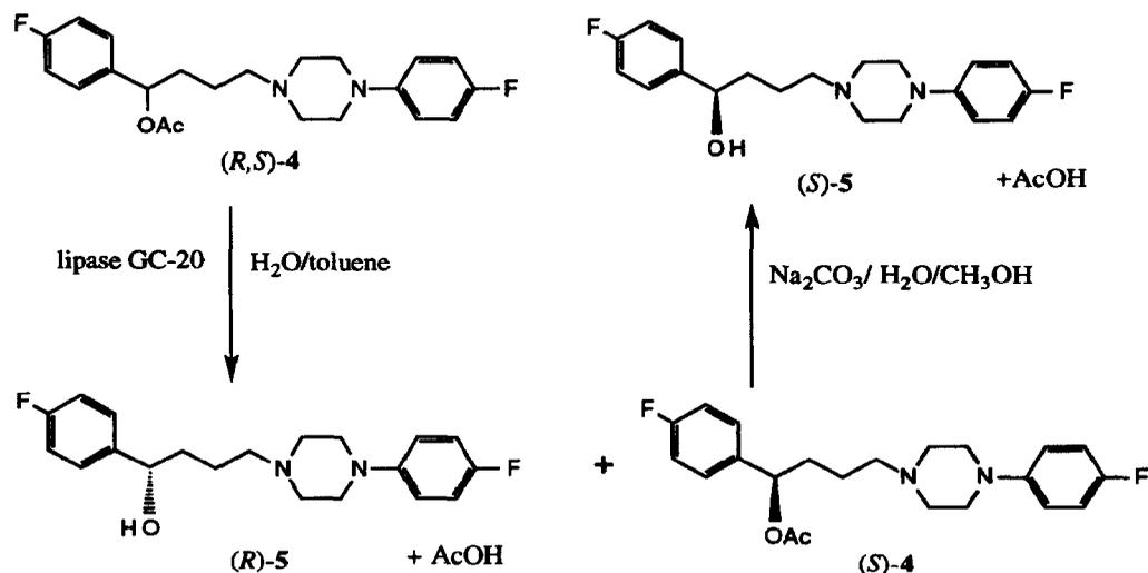
Figure 3. Resolution of  $\alpha$ -(4-fluorophenyl)-4-(5-fluoro-2-pyrimidinyl)-1-piperazinebutanol (**5**) using lipase GC-20.
