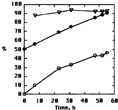
Figure 2. Time course of resolution of 1. Acetylation of 100 g 1 using lipase PS30 and isopropenyl acetate in heptane was carried out as described in EXPERIMENTAL. o, % conversion; ●, optical purity of 1 (% *S*); ▽, optical purity of 2 (% *R*).
