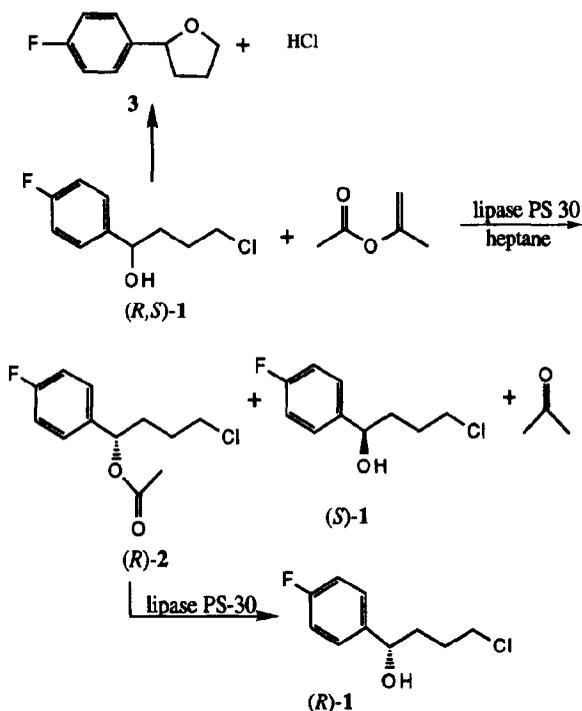
Figure 1. Resolution of  $\alpha$ -(3-chloropropyl)-4-fluorobenzene-methanol (**1**) using lipase PS30.
