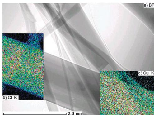
**Fig. 2** (a) TEM BF image of fibers obtained from TSC and cupric chloride. (b) STEM image of chlorine. (c) STEM image of copper.
