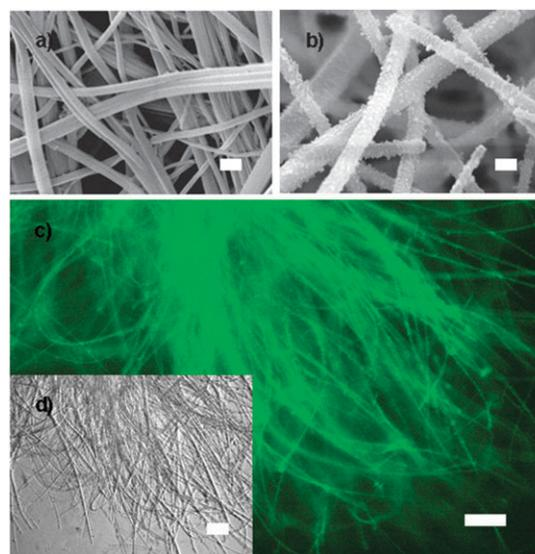
**Fig. 3** (a) SEM micrograph of fibers obtained from TSC and zinc chloride (scale bar = 1  $\mu\text{m}$ ). (b) SEM micrograph of fibers based on TSC and zinc chloride after radical polymerization in the presence of fluorescein methacrylate (scale bar = 1  $\mu\text{m}$ ). Optical micrographs of the same fibers under (c) blue light ( $\lambda = 485 \text{ nm}$ , scale bar = 100  $\mu\text{m}$ ) and (d) white light (scale bar = 100  $\mu\text{m}$ ).
