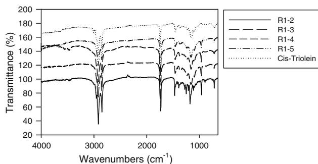
**Fig. 3** FTIR of metathesized triolein products. The structures of samples are shown in Scheme 3
