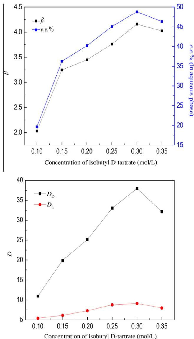
**Figure 4.** Influence of the initial concentration of *D*-IBTA on the distribution behavior. Initial concentration of *rac*-CHMA and SDS: 0.30 mg/mL and 0.50 mg/mL, pH 3.8, reflux time 4 h, and temperature 20 °C.
