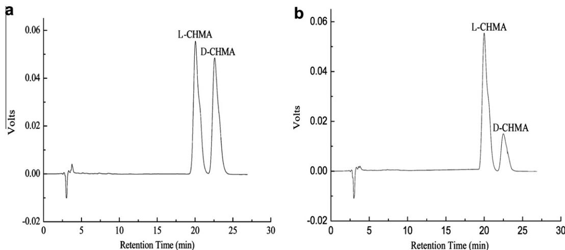
Figure 8. HPLC chromatograms of D,L-CHMA: (a) before and (b) after solvent sublation.
