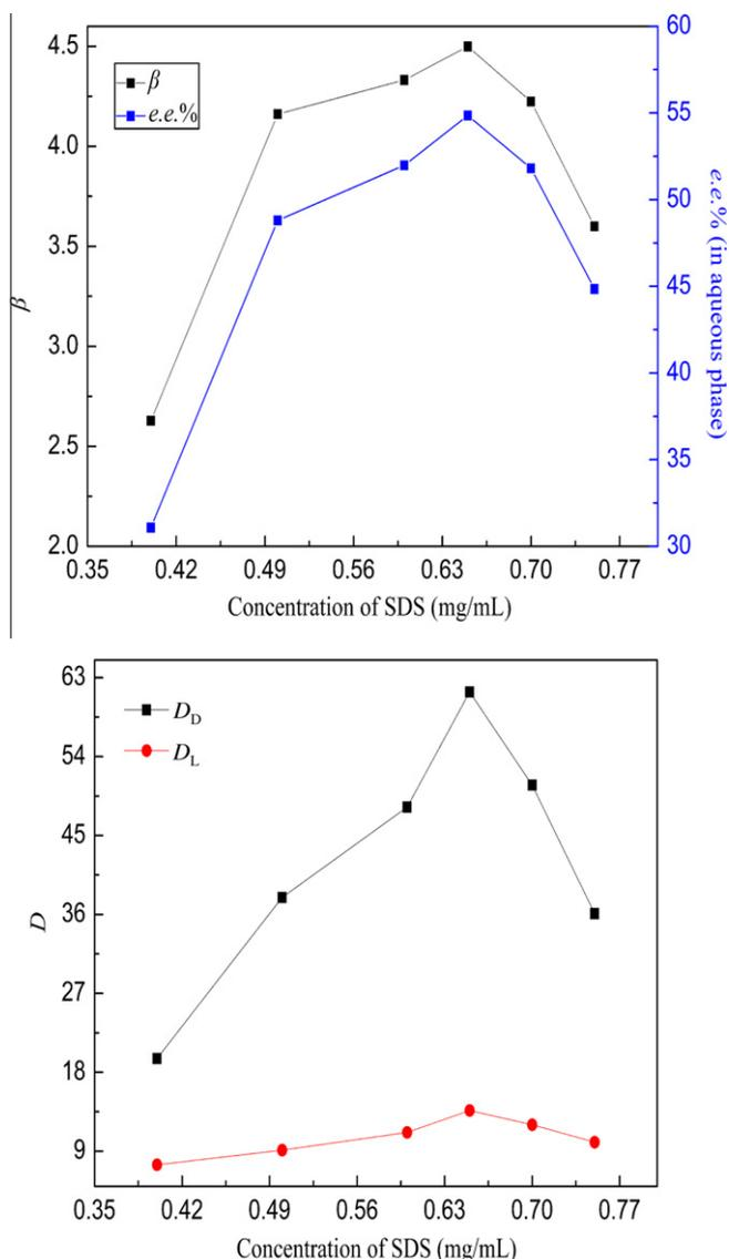
**Figure 5.** Influence of the concentration of SDS on the distribution behavior. Initial concentration of *rac*-CHMA and *D*-IBTA: 0.30 mg/mL and 0.30 mol/L, pH 3.8, reflux time 4 h, and temperature 20 °C.
