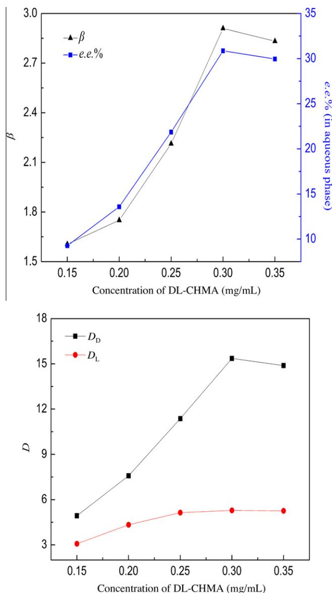
**Figure 2.** Influence of the initial concentration of *rac*-CHMA on the distribution behavior. Initial concentration of *D*-IBTA and SDS: 0.20 mol/L and 0.50 mg/mL, pH 3.2, reflux time 4 h and temperature 20 °C.
