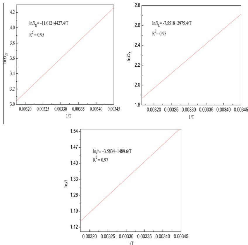
**Figure 6.** Influence of the temperature on the distribution behavior. Initial concentration of *rac*-CHMA, *D*-IBTA, and SDS: 0.30 mg/mL, 0.30 mol/L, and 0.65 mg/mL, pH 3.8, reflux time 4 h.
