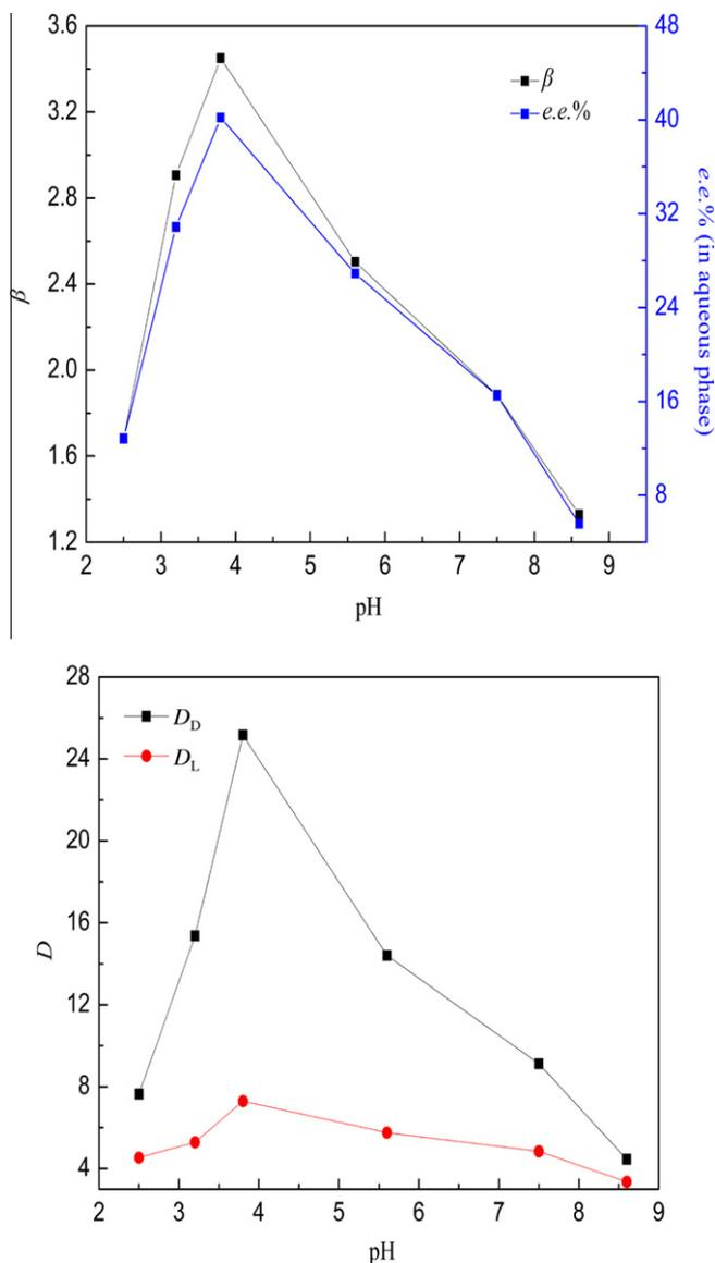
**Figure 3.** Influence of the pH on the distribution behavior. Initial concentration of *rac*-CHMA, *D*-IBTA, and SDS: 0.30 mg/mL, 0.20 mol/L, and 0.50 mg/mL, reflux time 4 h and temperature 20 °C.
