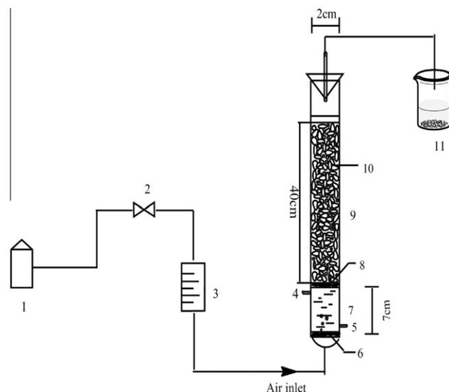
**Figure 7.** Schematic showing the apparatus used in this work. (1) Air pump, (2) control valve, (3) rotameter, (4) inlet for solution, (5) outlet for solution, (6) gas distributor, (7) sample pool, (8) microporous plate, (9) glass column, (10) ceramic ring and (11) bubble receiver.
