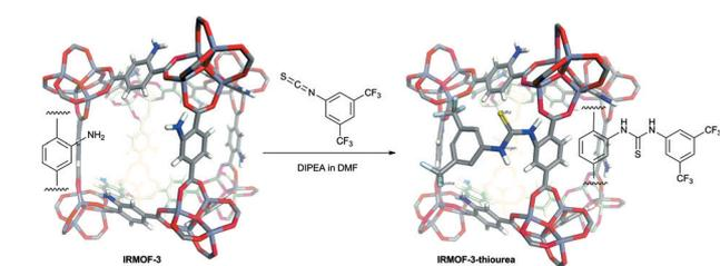
Scheme 1 Post-synthetic modification of IRMOF-3 with 3,5-bis(trifluoromethyl)phenyl isothiocyanate.
