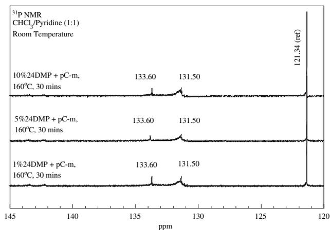
**Fig. 7.**  $^{31}\text{P}$  NMR of product from *pC*-m initiated by 1, 5 and 10% by mole of 2,4-dimethylphenol (24DMP) at 160 °C for 30 min (Exp. D) and derivatized with 132-DOP (Scheme 2) in chloroform and pyridine at room temperature.
