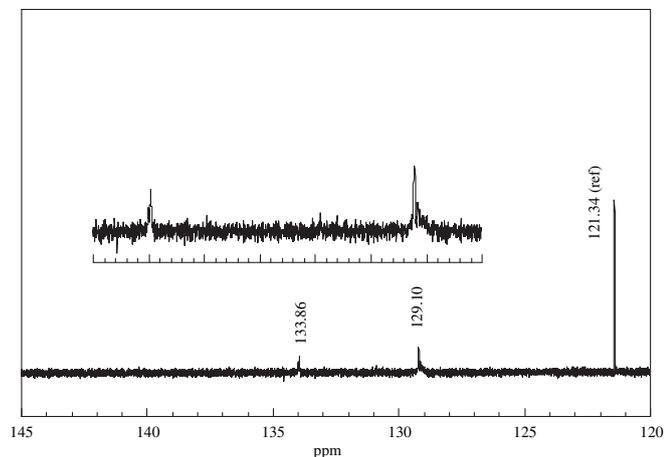
**Fig. 8.**  $^{31}\text{P}$  NMR spectrum of not fully cured (Exp. E, Table 1) bisphenol-A and methylamine based benzoxazine.
