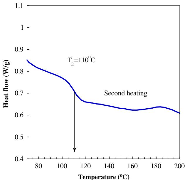
Fig. 3. Second DSC run of the piperazine-based poly(Mannich base).
