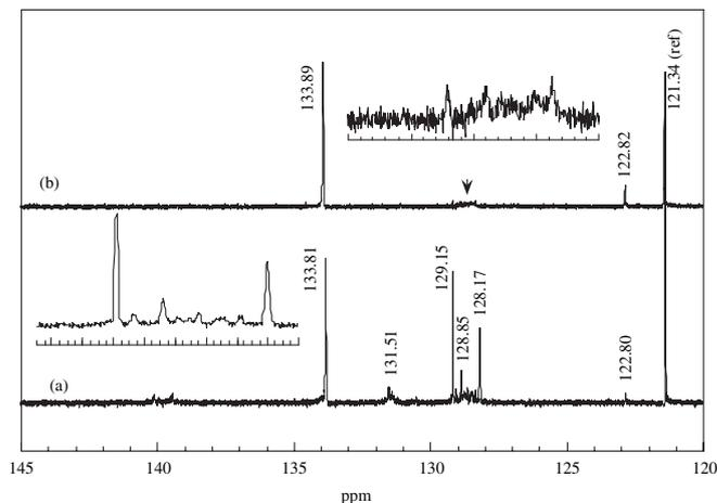
Fig. 5. <sup>31</sup>P NMR spectra of (a) product from Exp. A (Table 1); and (b) product from Exp. B (Table 1).
