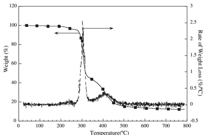
**Fig. 2.** TGA thermogram and derivative of weight loss of polymer product from polycondensation of *p*-Cresol, formaldehyde, and piperazine.
