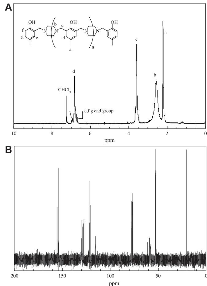
**Fig. 1.** (A)  $^1\text{H}$  and (B)  $^{13}\text{C}$  NMR of polymer product from polycondensation of *p*-cresol, formaldehyde, and piperazine.
