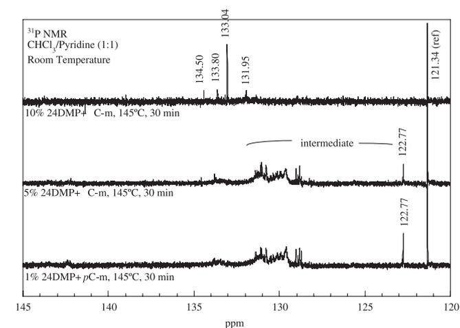
**Fig. 6.**  $^{31}\text{P}$  NMR spectra of product from *pC*-m initiated by 1, 5 and 10 mol% of 2,4-dimethylphenol (24DMP) at 145 °C for 30 min (Exp. C) and derivatized with 132-DOP (Scheme 2) in chloroform and pyridine at room temperature.
