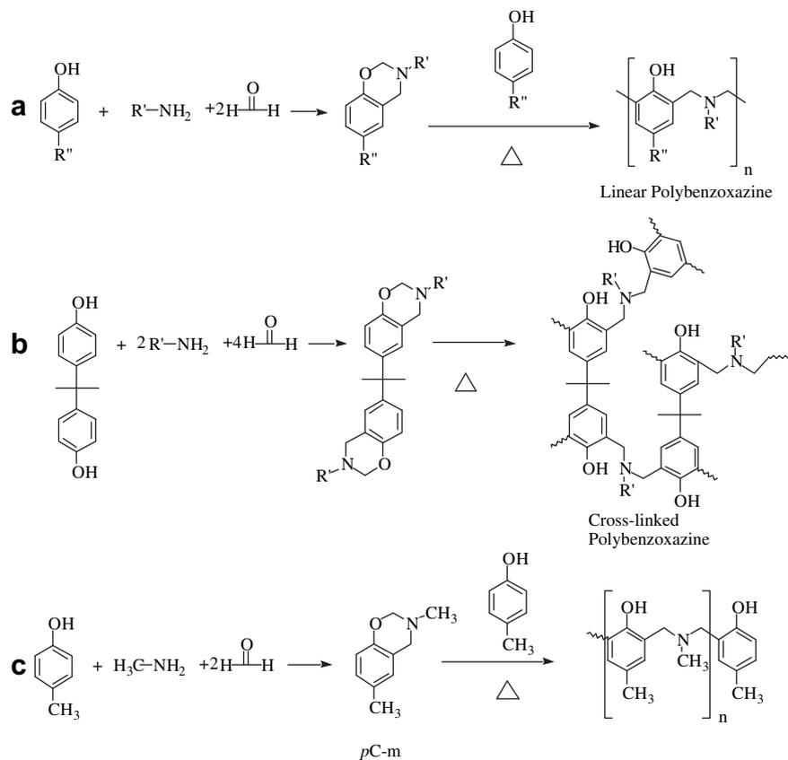
**Scheme 1.** (a) Synthesis of linear polybenzoxazine (b) synthesis of cross-linked polybenzoxazine (c) *p*-cresol, methylamine based benzoxazine (*pC-m*) synthesis and expected reaction product ( $R'$ , and  $R''$  are substituents).
