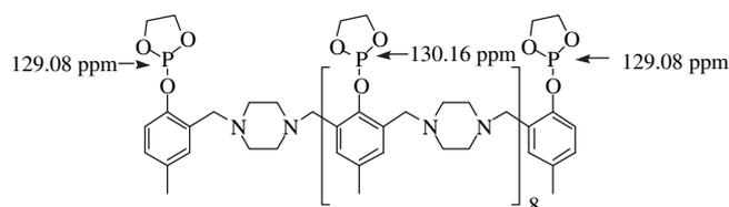
**Scheme 5.**  $^{31}\text{P}$  NMR resonance of Mannich polymer from the reaction between *p*-cresol, formaldehyde, and piperazine.
