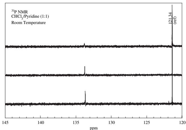
**Fig. 9.**  $^{31}\text{P}$  NMR spectrum of crude products from polymerization of bisphenol methylamine based benzoxazine at 185 °C for 10, 45, and 60 min from lower to upper spectrum.
