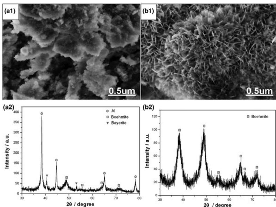
**Fig. 3.** FESEM micrographs and XRD patterns of the hydrolysis products from 8 h ball-milled (a) Al and (b) Al-13 wt% Ce composite.
