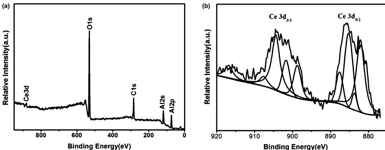
Fig. 2. (a) XPS survey spectrum and (b) high-resolution Ce 3d spectra of Al-13 wt% Ce.
