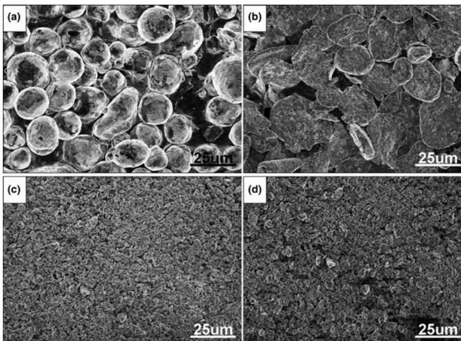
Fig. 5. FESEM micrographs of (a) un-milled Al, Al-13 wt% Ce after ball-milling for (b) 1 h, (c) 8 h, and (d) 12 h.
