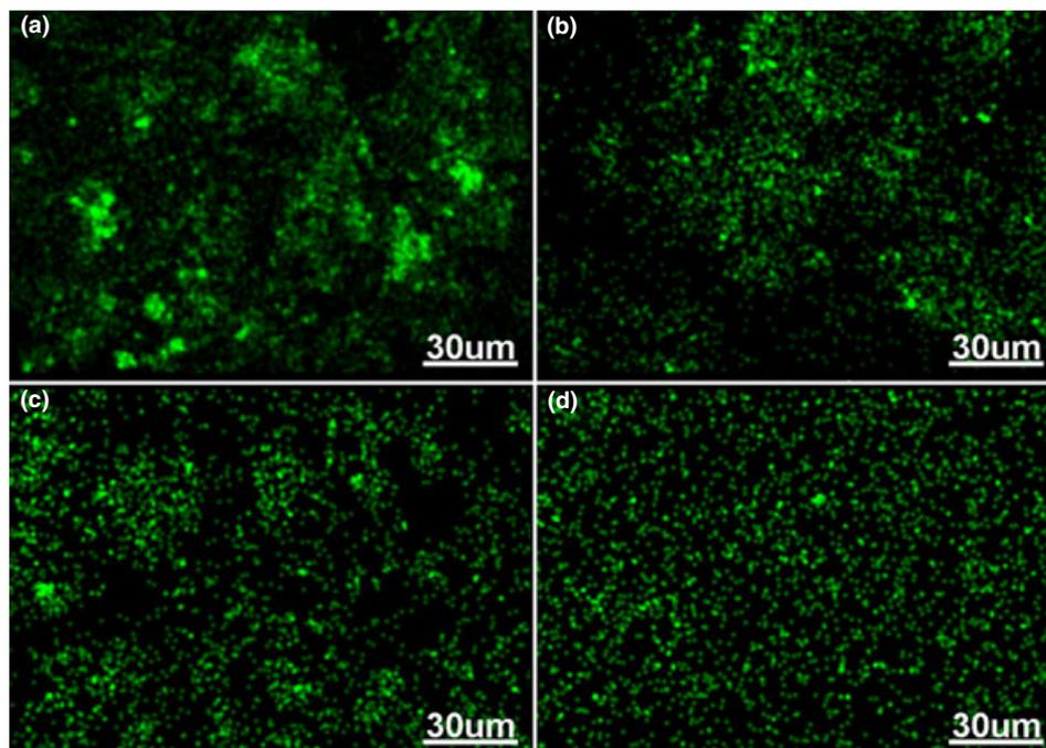
Fig. 6. EDX mapping of Ce in Al-13 wt% Ce composite materials as a function of the milling time: (a) 1 h, (b) 5 h, (c) 8 h, and (d) 10 h.
