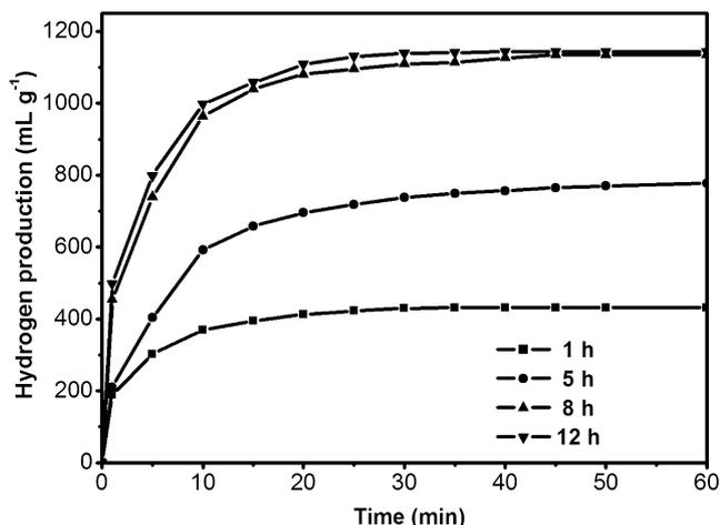
Fig. 4. The hydrogen production curves of Al-13 wt% Ce after different ball-milling times.
