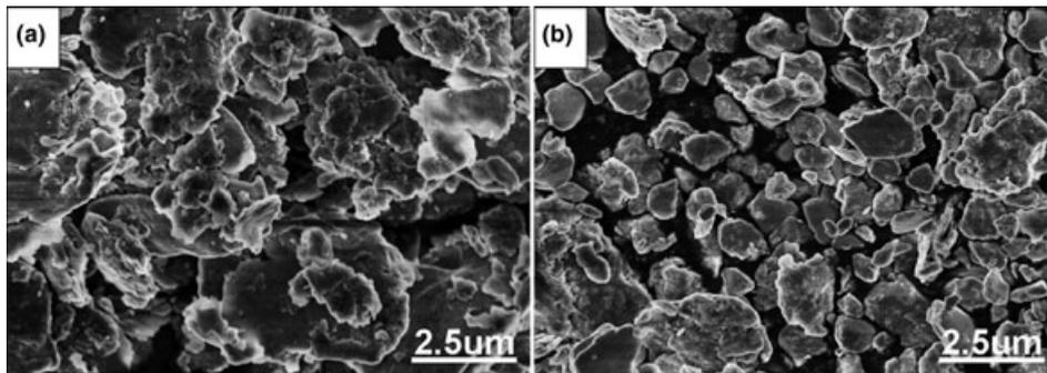
Fig. 8. FESEM micrographs of 8 h ball-milled (a) Al-5 wt% Ce and (b) Al-5 wt% Ce-10 wt% NaCl.
