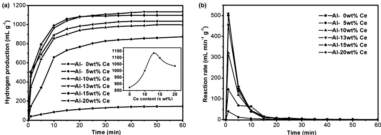
Fig. 1. The hydrogen production curves (a) and the reaction rate curves (b) of 8 h ball-milled Al-*x* wt% Ce composites with pure water.
