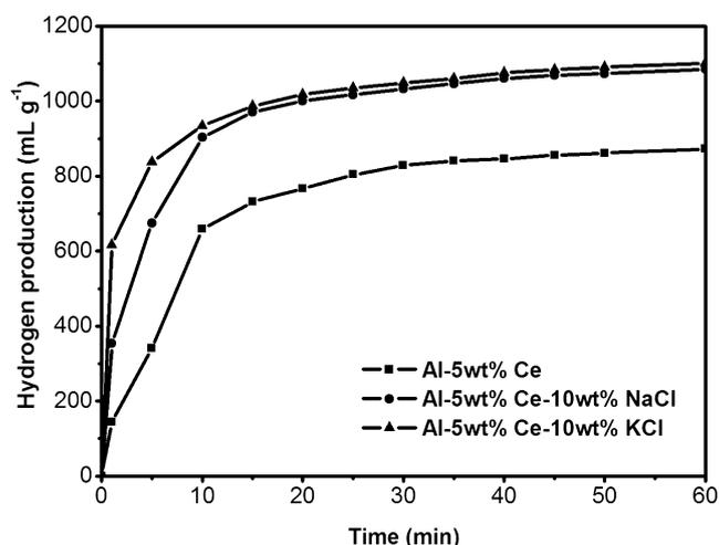
Fig. 7. The hydrogen production curves of 8 h ball-milled Al-5 wt% Ce-10 wt% alkali chloride with pure water.
