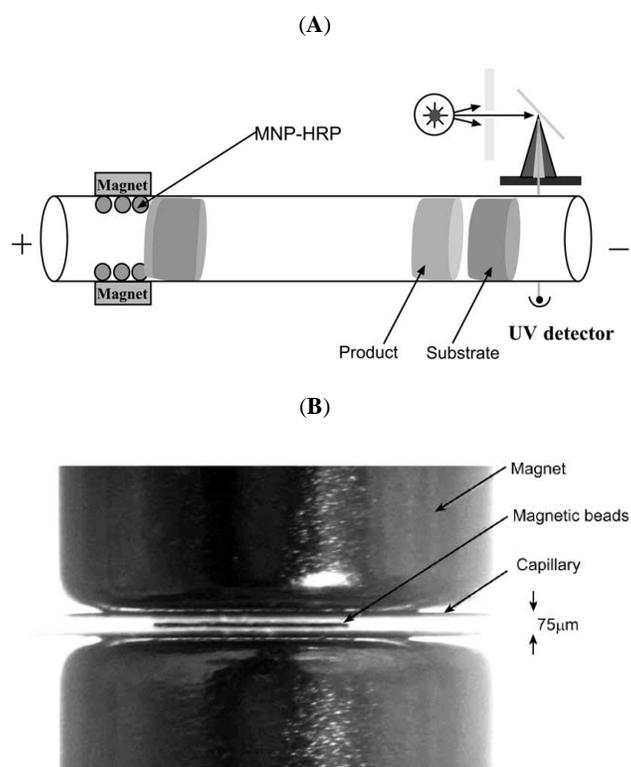
**Fig. (1).** (A) Schematic illustration of the EMMA device used for biotransformation studies. (B) Optical image of a microreactor after packing with magnetic nanoparticles (MNPs).
