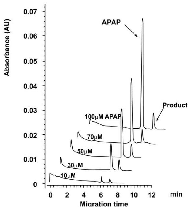
**Fig. (2).** Electropherograms of in-capillary reactions at concentrations of APAP between 10-100 $\mu$ M. Separation conditions: background electrolyte 12.5mM PB (pH 7.4), separation current 90 $\mu$ A (18kV), detection at 245 nm, temperature of capillary 25 $^{\circ}$ C. Injection: 1mg/ml HRP-MNPs in PB; hydrodynamic mode for 3s, APAP in PB (12.5mM) and sulfated- $\beta$ -CD(20mg/ml); electrokinetic mode 18kV for 10s.
