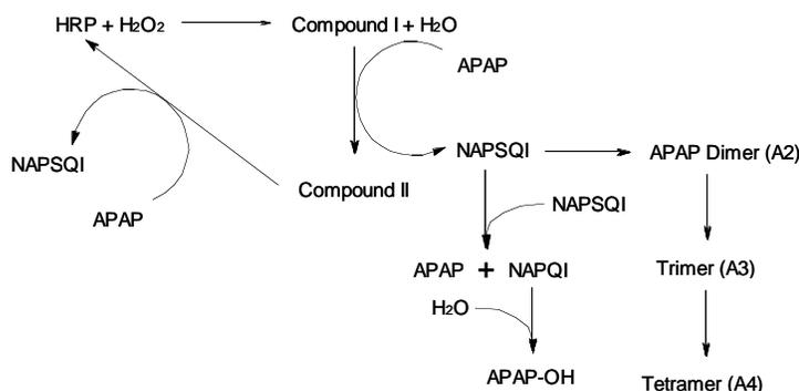
**Scheme 2.** Biotransformation pathway of paracetamol (APAP) in the HRP-MNPs/H<sub>2</sub>O<sub>2</sub> suspension at pH 7.4.
