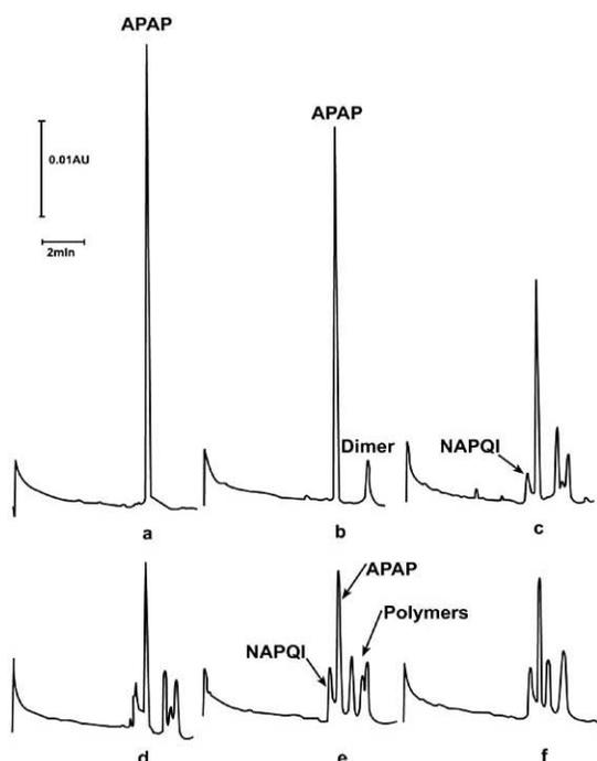
**Fig. (4).** Off-line biotransformation studies. [APAP]=10<sup>-4</sup>M, 20 μl of HRP-NPMs [H<sub>2</sub>O<sub>2</sub>] = 10<sup>-4</sup>M. Reaction time a: 0 min b: 1 min, c: 10 min, d: 20 min, e:30 min, f:50 min.
