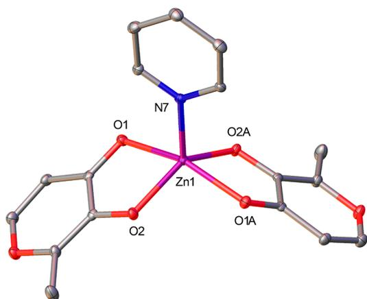
**Figure 2.** Molecular structure of  $[\text{Zn}(\text{MalO})_2(\text{py})]$  (**2**). The displacement ellipsoids are drawn at the 30% probability level. Hydrogen atoms are omitted for clarity. Selected bond lengths (Å) and angles (deg): Zn1–O1 2.140(2), Zn1–O2 1.980(2), Zn1–N7 2.034(3), O1–Zn1–O1A 160.3(3), O1–Zn1–O2 81.2(3), O1–Zn1–O2A 91.5(3), O2–Zn1–O2A 137.1(3), O1–Zn1–N7 100.1(2), O2–Zn1–N7 111.5(2).
