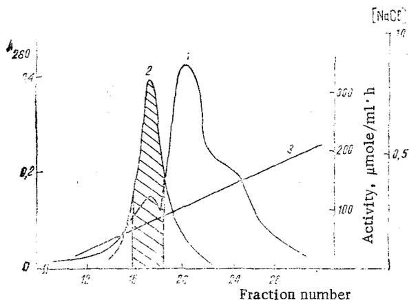
Fig. 3. Chromatography of an acylase preparation on a column of DEAE-cellulose at pH 5.7. Symbols the same as in Fig. 1.
