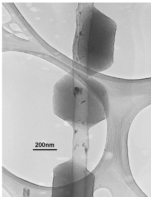
Fig. 3. TEM image of MCM-CNT composite after calcination in air for the elimination of CNT.
