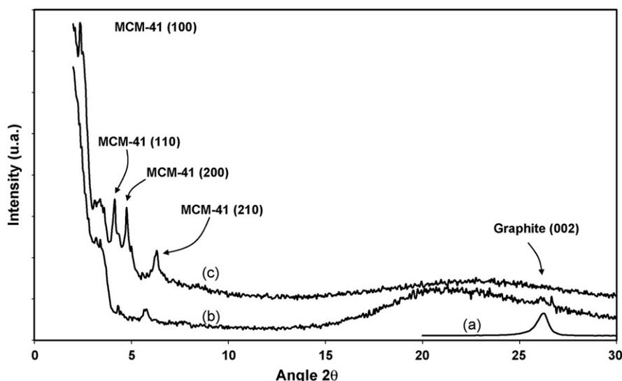
Fig. 2. X-ray diffraction pattern of carbon nanotubes as obtained by spray pyrolysis synthesis (a), MCM-CNT after filtration and washing (b) and MCM after calcination (c).
