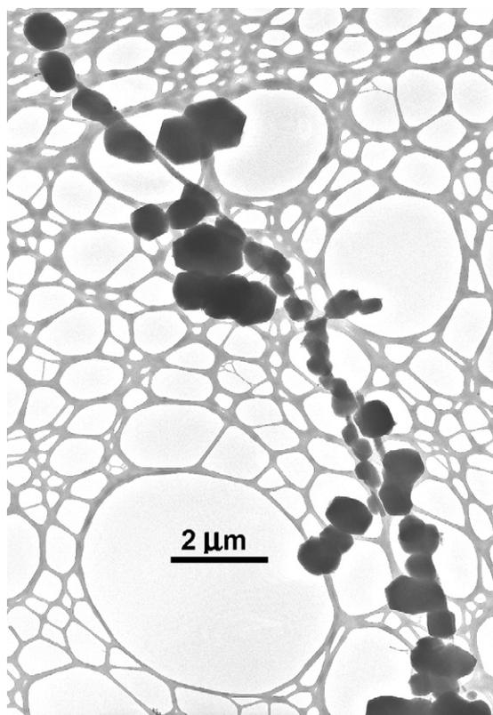
Fig. 1. MCM-41 particles forming a necklace structure by interconnection with carbon nanotubes.
