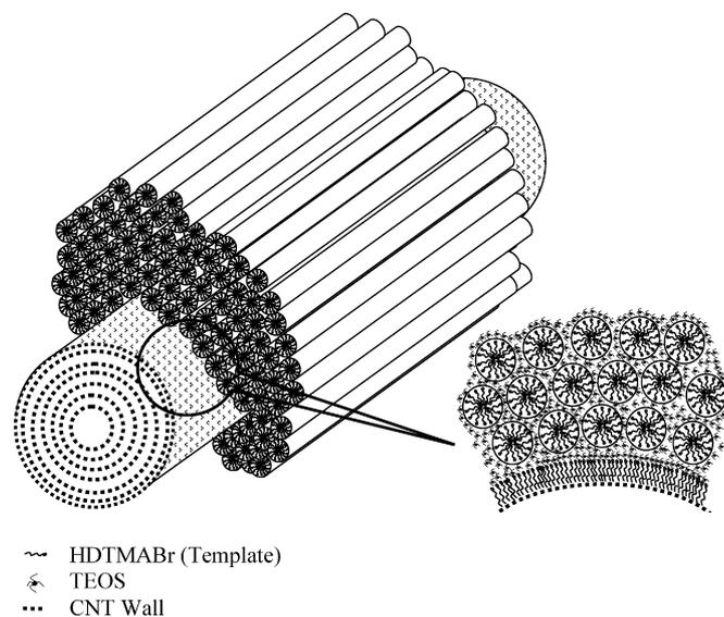
Fig. 5. Schematic representation of the arrangement of reactives during the synthesis of the MCM/CNT composite. Hydrophobic part of template has affinity with the CNT walls, so organization of template on CNT surface becomes similar to the other surface of template micelles. TEOS surrounds the hydrophilic surfaces around covered CNT and rod like micelles. CNT align in the same way of rod micelles.
