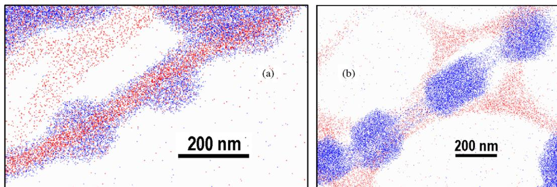
Fig. 4. Micrographs of MCM-41 particles interconnected by carbon nanotubes. (a) STEM mapping image overlay of carbon (red) and silicon (blue) before calcination. (b) STEM mapping image after calcination of nanocomposite in air; since the walls of nanotubes were covered by  $\text{SiO}_2$ , the structure of interconnected particles remains in spite of the burning of carbon.
